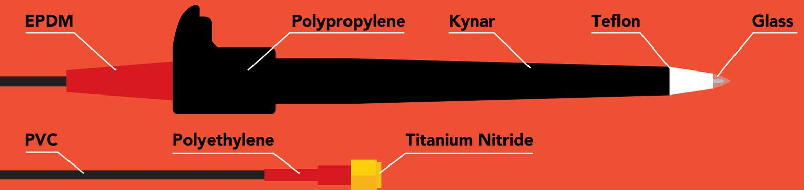
This pH probe can be **fully submerged** in fresh or salt water, up to the SMA connector **indefinitely**.
