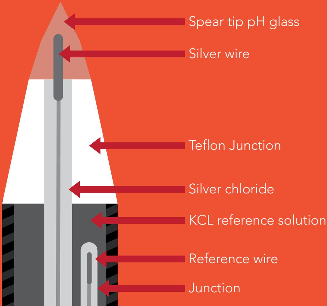
A pH electrode is a passive device that detects a current generated from hydrogen ion activity. This current (*which can be positive or negative*) is very weak and cannot be detected with a multimeter, or an analog to digital converter. This weak electrical signal can easily be disrupted and care should be taken to only use proper connectors and cables.
