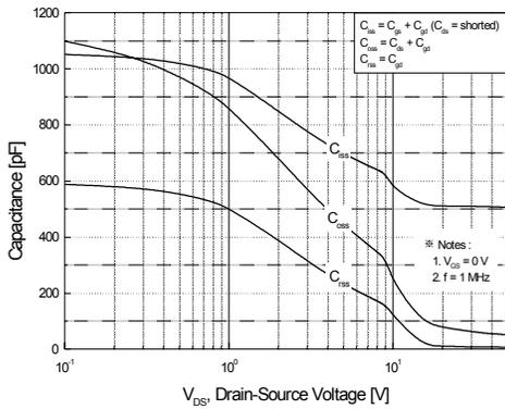
Figure 5. Capacitance Characteristics
