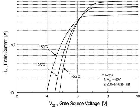
Figure 2. Transfer Characteristics
