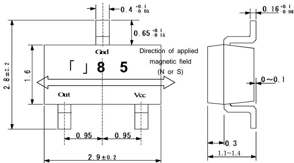
Coplanarity : less than 0.1mm(including under reflow condition)
