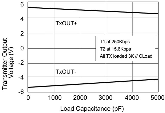
**Figure 2: Transmitter Output Voltage vs. Load Capacitance**
