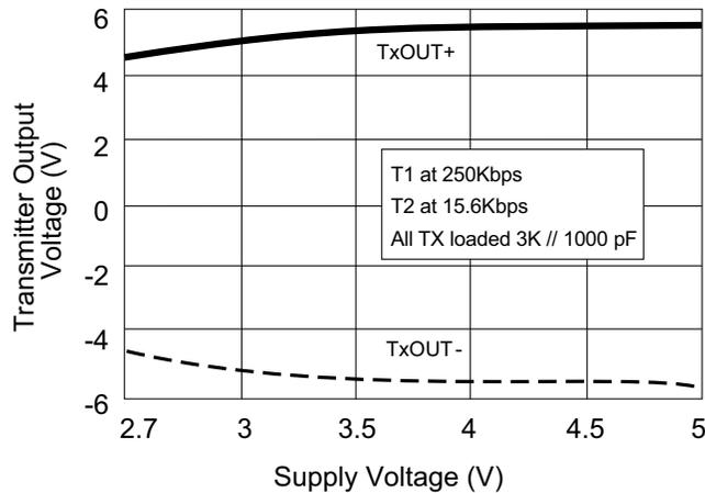
**Figure 6: Transmitter Output Voltage vs. Supply Voltage**
