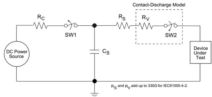
**Figure 19: ESD Test Circuit for IEC61000-4-2**
