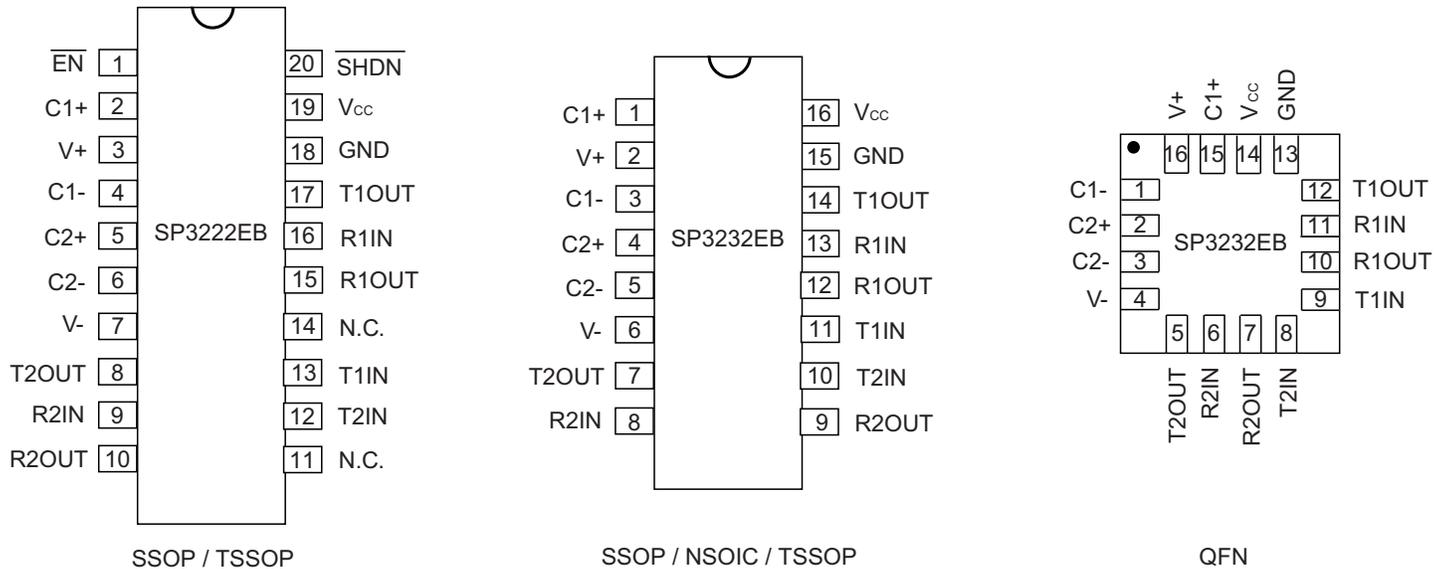
**Figure 7: Pinout Configurations for the SP3222EB and SP3232EB**
