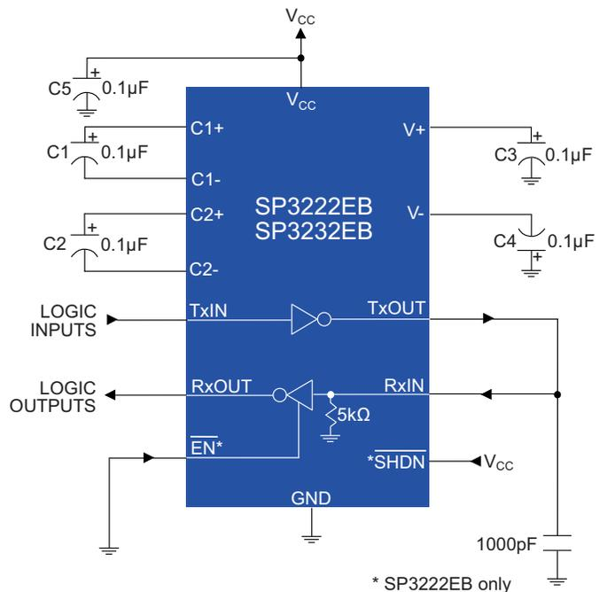
**Figure 10: SP3222EB / SP3232EB Driver Loopback Test Circuit**
