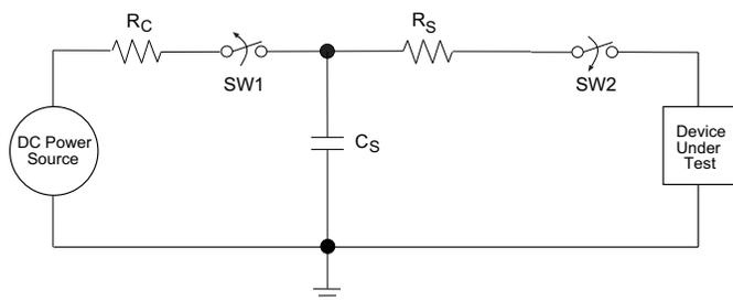
**Figure 18: ESD Test Circuit for Human Body Model**
