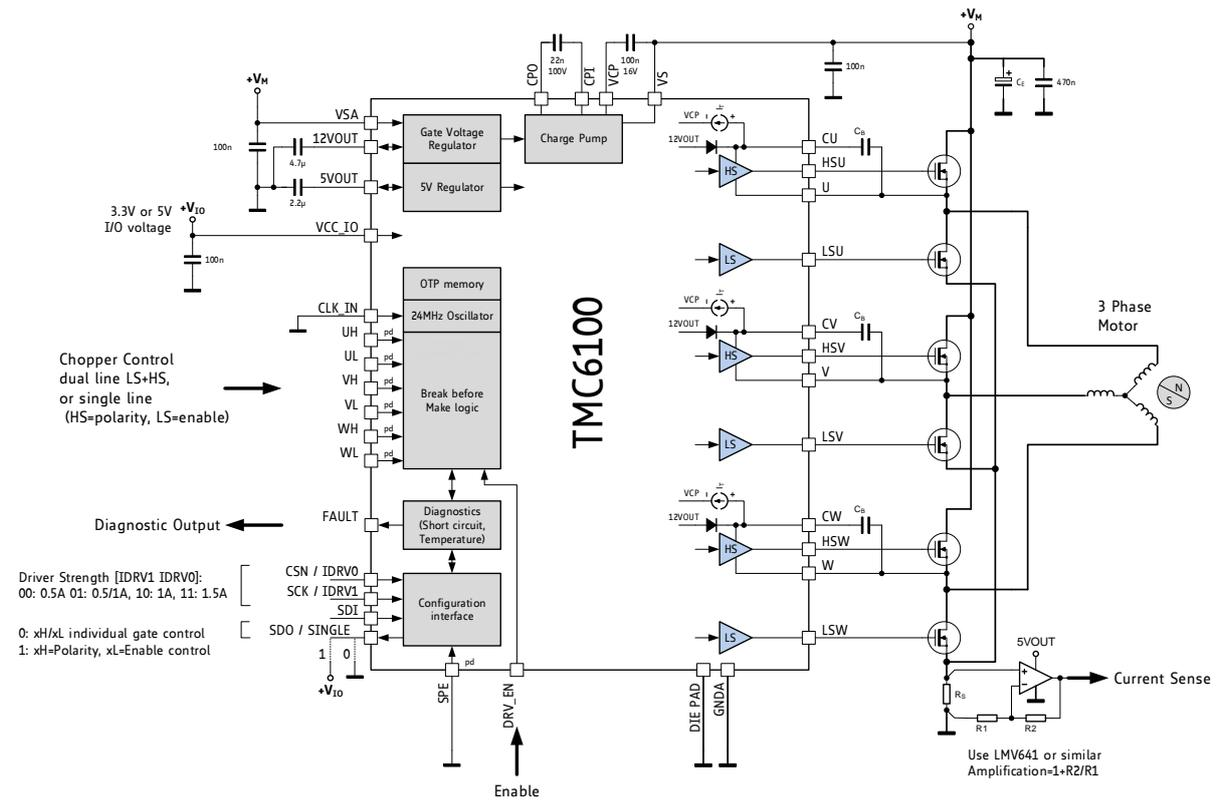
Figure 1.2 Standalone application using single shunt current sensing
