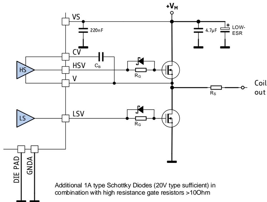
**Figure 3.10 Diodes for safe off condition with high gate series resistance**
