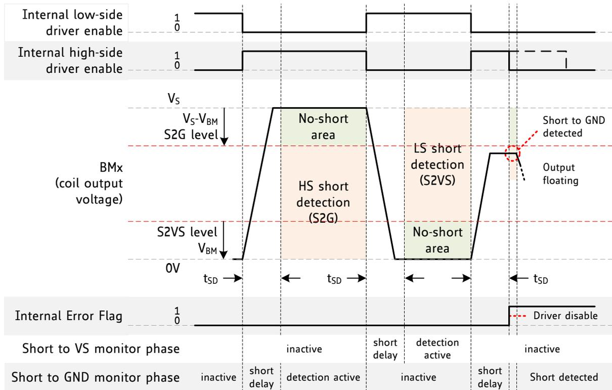
**Figure 6.1 Short detection (U, V or W output)**
