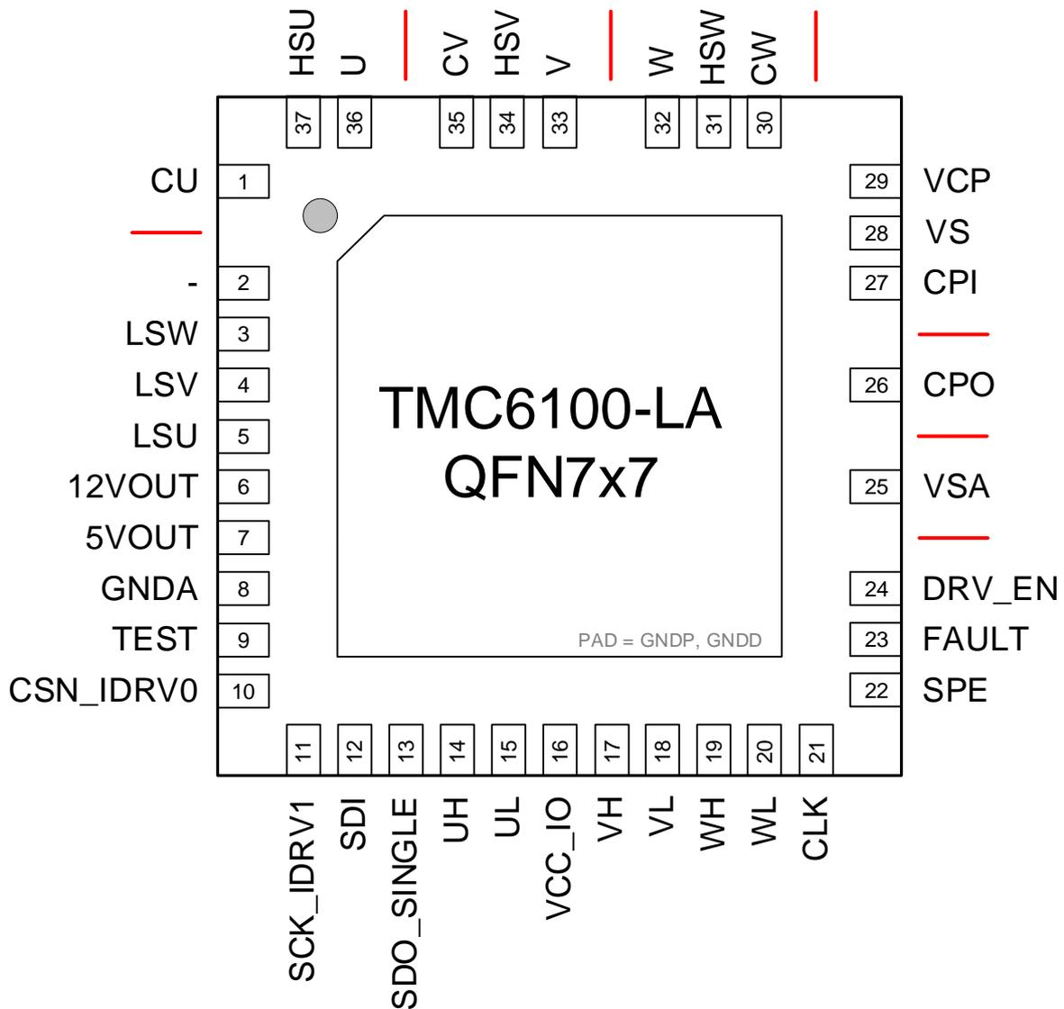
Figure 2.1 TMC6100-LA pinning QFN 37 special (7x7mm<sup>2</sup>)
