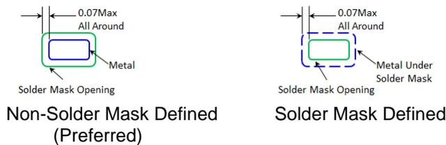
**Figure 11 Solder Mask Pattern**
