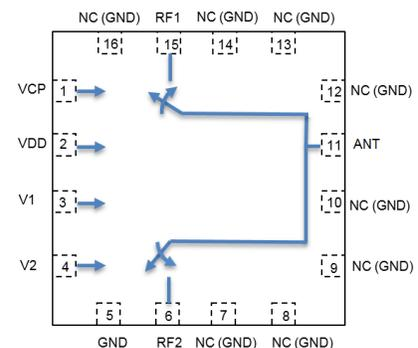
**Figure 2 Function Block Diagram**
