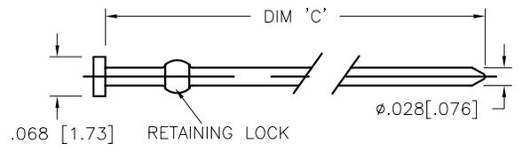
FIG. 1 RETENTION ROD DETAIL
