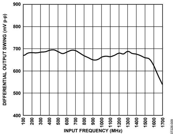
Figure 9. LVDS Differential Output Swing vs. Input Frequency
