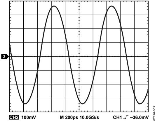
Figure 3. LVDS Output Waveform at 1200 MHz
