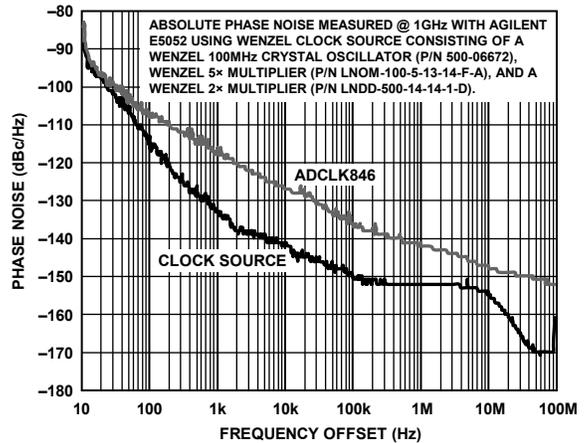
Figure 12. Absolute Phase Noise LVDS at 1000 MHz
