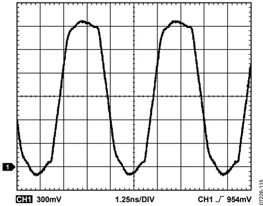
Figure 15. CMOS Output Waveform at 200 MHz, 10 pF Load
