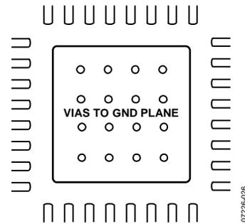
Figure 23. PCB Land Example for Attaching Exposed Paddle
