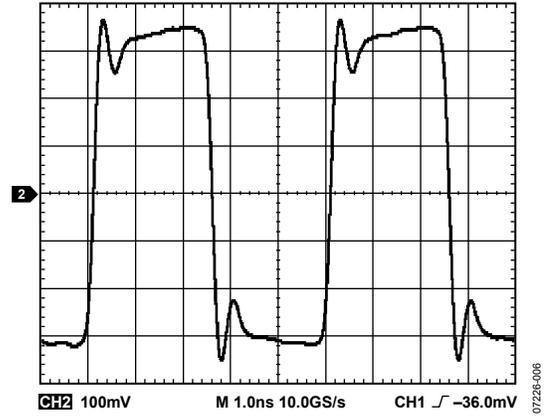
Figure 6. LVDS Output Waveform at 200 MHz
