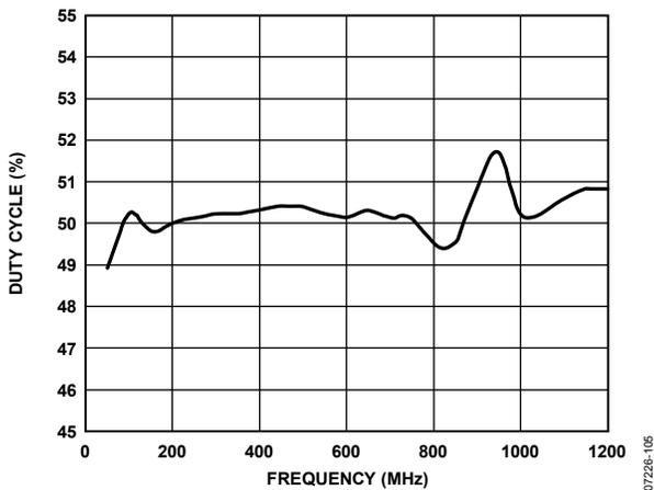
Figure 5. LVDS Output Duty Cycle vs. Frequency
