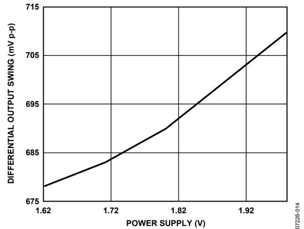
Figure 8. LVDS Output Swing vs. Power Supply Voltage
