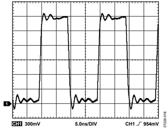
Figure 18. CMOS Output Waveform at 50 MHz, 10 pF Load
