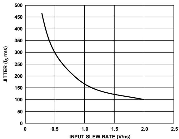
Figure 11. Additive Broadband Jitter vs. Input Slew Rate
