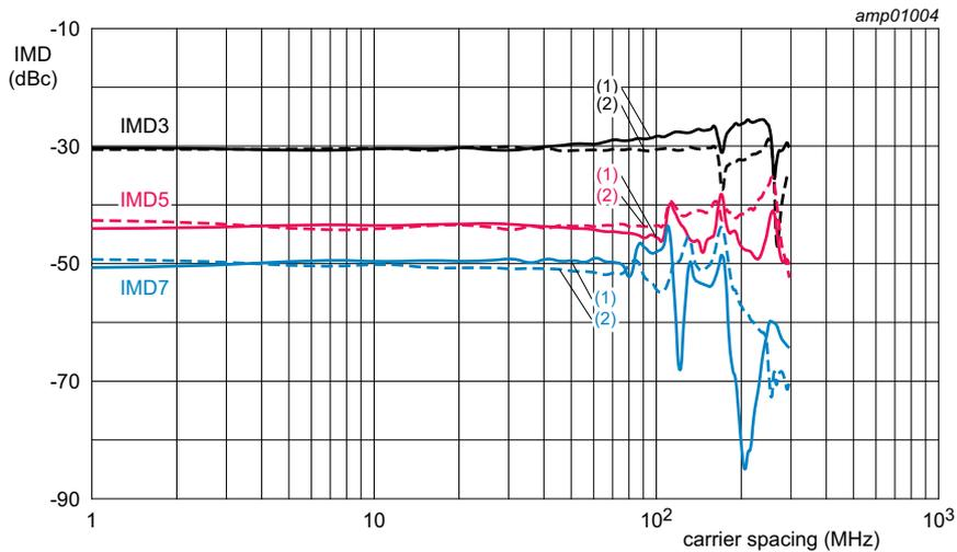
$V_{DS} = 28\text{ V}$ ;  $V_{GS(amp)peak} = V_{GS(amp)main} - 0.55\text{ V}$ ;  $I_{Dq} = 20\text{ mA}$ ;  $f = 2600\text{ MHz}$ .
