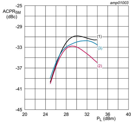
$V_{DS} = 28\text{ V}$ ;  $V_{GS(amp)peak} = V_{GS(amp)main} - 0.55\text{ V}$ ;  $I_{Dq} = 20\text{ mA}$ .
