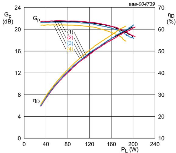
$V_{DS} = 28 \text{ V}; I_{Dq} = 1200 \text{ mA}; t_p = 10 \mu\text{s}; \delta = 10 \%$ .
