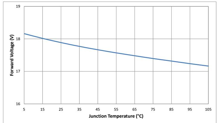
**CXM-7, 9V Optical & Electrical Characteristics**
