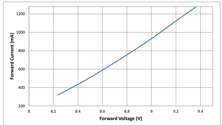
**CXM-7, 9V Optical & Electrical Characteristics**
