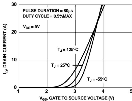
**Figure 5. Transfer Characteristics**
