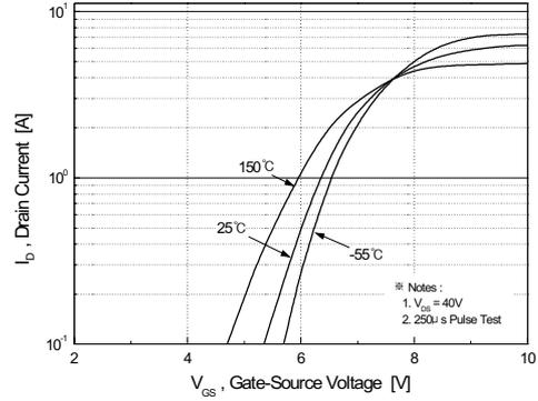
Figure 2. Transfer Characteristics
