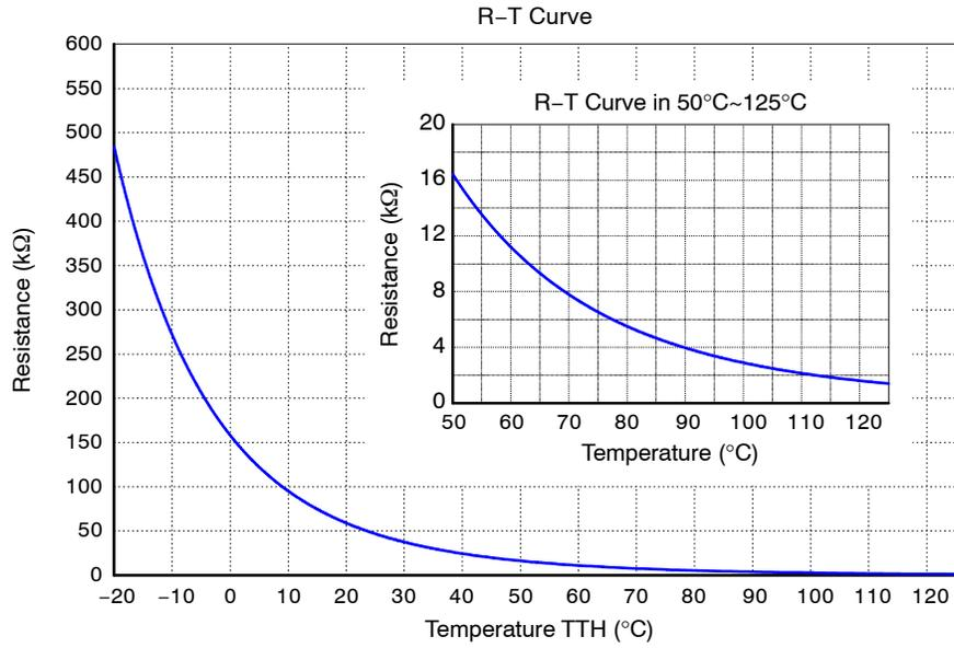
Figure 5. R-T Curve of The Built-In Thermistor
