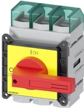
SENTRON, Switch disconnecter 3LD, emergency switching-off switch, 3-pole,  $I_u=250$  A, operating power / at AC-23 A 400 V: 132 kW, front-mounted, knob-operated mechanism, red/yellow, 4-hole mounting of the handle
