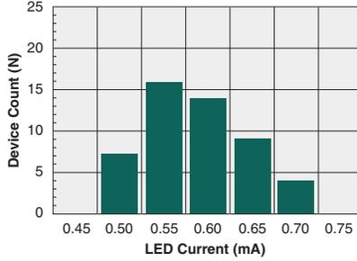
**Typical  $I_F$  for Switch Dropout**
