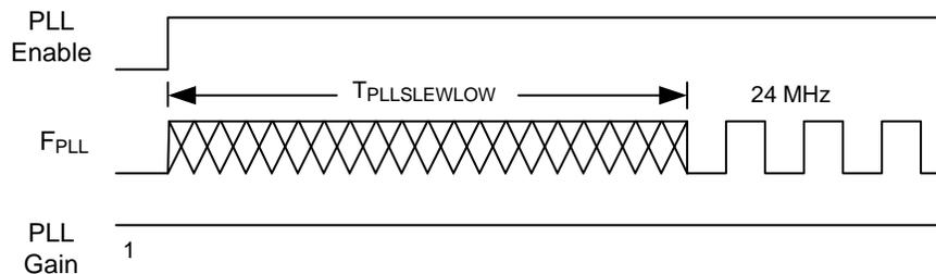
Figure 9. External Crystal Oscillator Startup Timing Diagram
