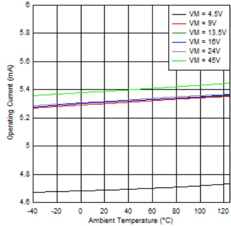
**Figure 6-4. Operating Current over Temperature**
