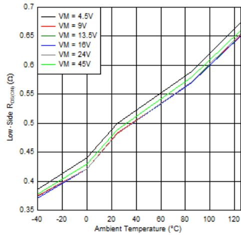
**Figure 6-6. Low-Side  $R_{DS(ON)}$  over Temperature**
