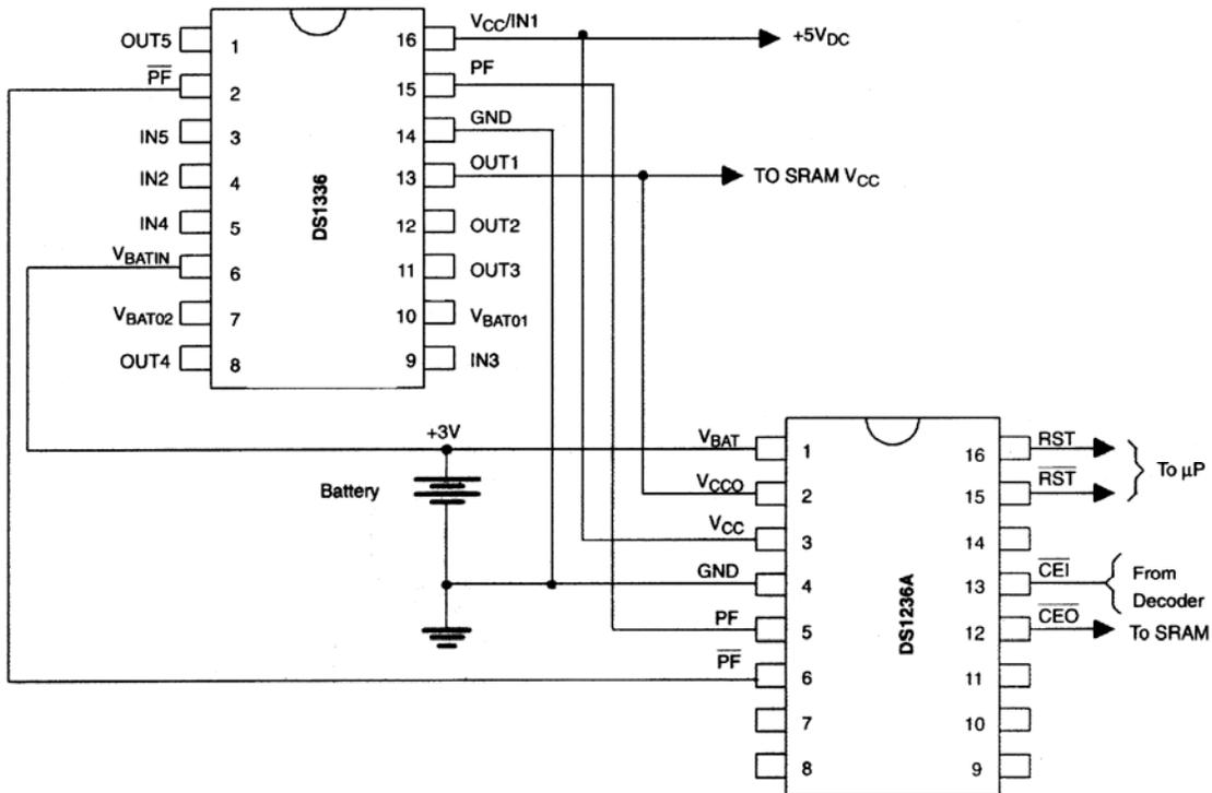
CMOS MODE POWER-DOWN (RC = V<sub>CC0</sub>) Figure 9
