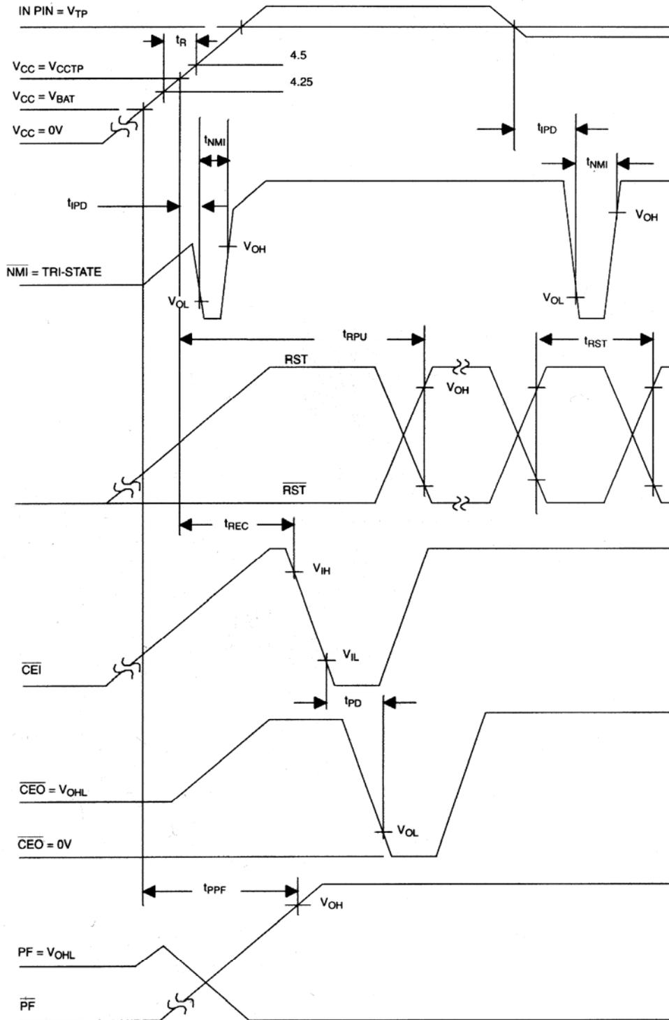
CMOS MODE POWER-UP (RC = V<sub>CC0</sub>) Figure 12
