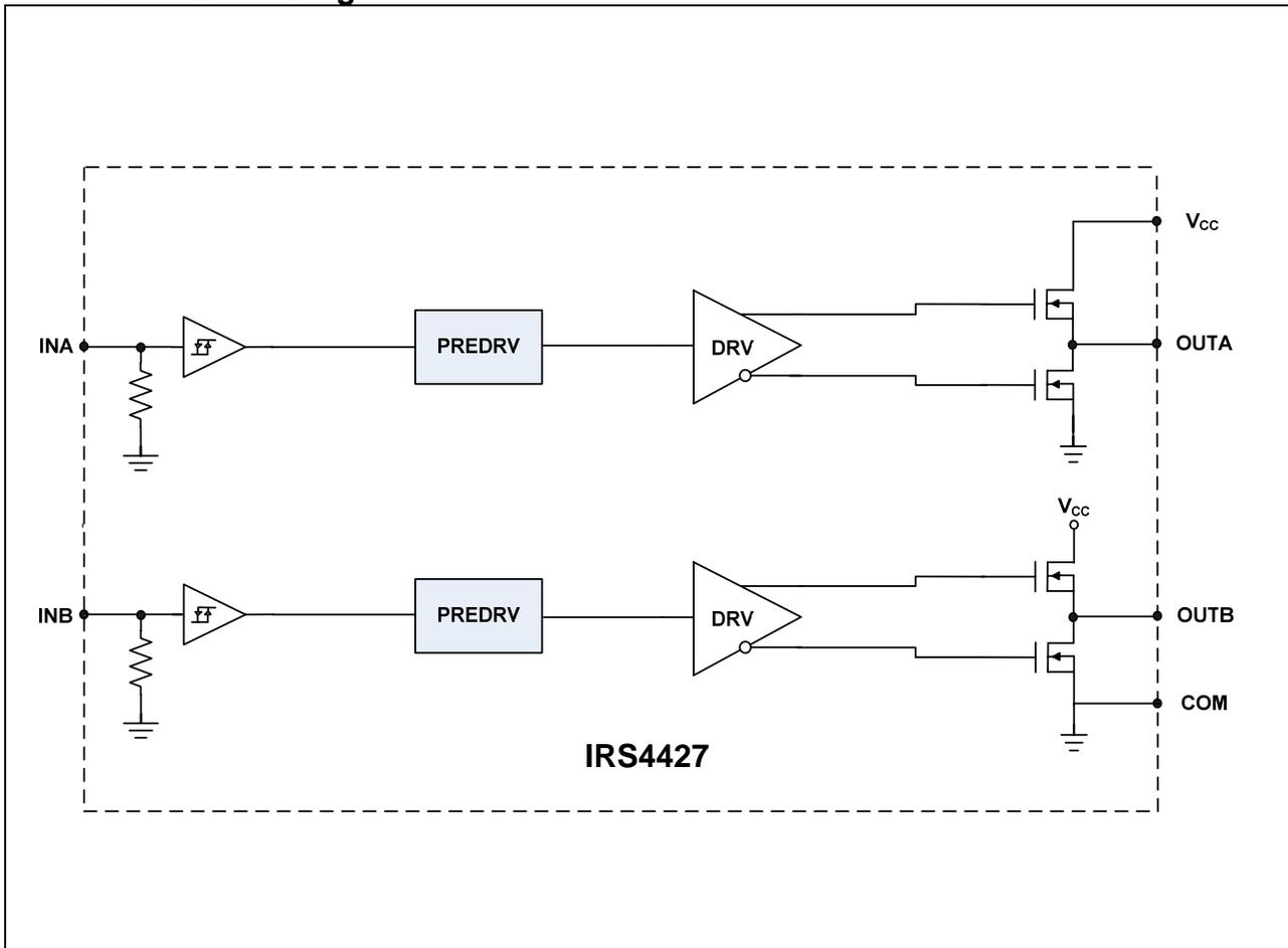
**Input/Output Pin Equivalent Circuit Diagrams**
