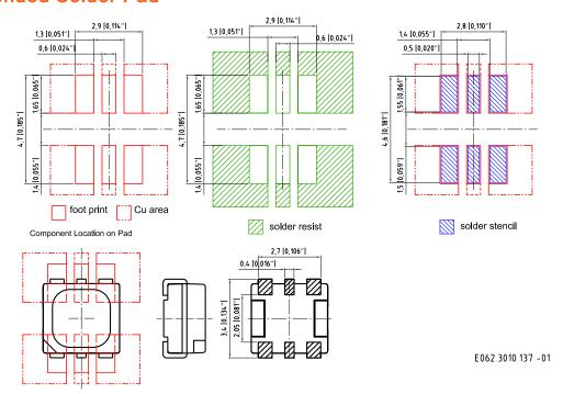
For superior solder joint connectivity results we recommend soldering under standard nitrogen atmosphere. Package not suitable for ultra sonic cleaning.
