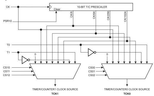
For Timer/Counters 0 and 1, the four prescaled selections are: CK/8, CK/64, CK/256, and CK/1024, where CK is the Oscillator clock. For the two Timer/Counters 0 and 1, CK, external source and stop can also be selected as clock sources. Setting the PSR10 bit in SFIOR Resets the prescaler. This allows the user to operate with a predictable prescaler. Note that Timer/Counter1 and Timer/Counter0 share the same prescaler and a Prescaler Reset will affect both Timer/Counters.
