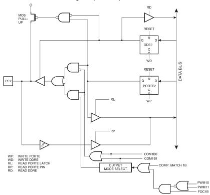
Figure 73. Port E Schematic Diagram (Pin PE2)
