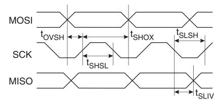
**Table 49.** Serial Programming Characteristics,  $T_A = -40^{\circ}\text{C}$  to 85°C,  $V_{CC} = 2.7 - 5.5\text{V}$  (unless otherwise noted)
