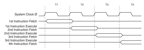
Figure 22 shows the internal timing concept for the Register File. In a single clock cycle an ALU operation using two register operands is executed and the result is stored back to the destination register.
