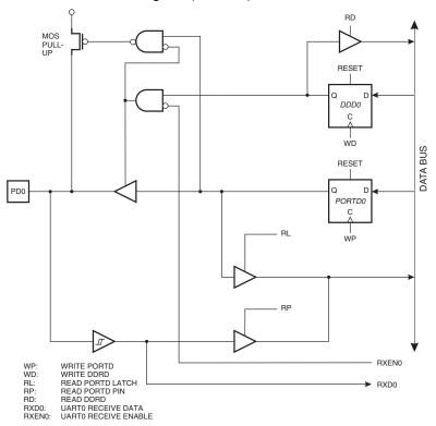
Figure 65. Port D Schematic Diagram (Pin PD1)
