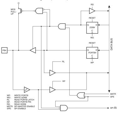
Figure 60. Port B Schematic Diagram (Pin PB5)
