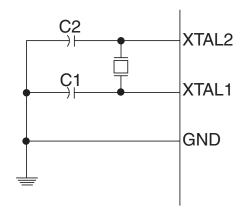
Figure 3. External Clock Drive Configuration
