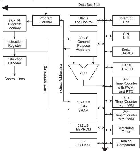
Figure 4. The ATmega161 AVR RISC Architecture
