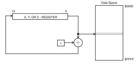
The X-, Y-, or Z-register is incremented after the operation. Operand address is the contents of the X-, Y-, or Z-register prior to incrementing.
