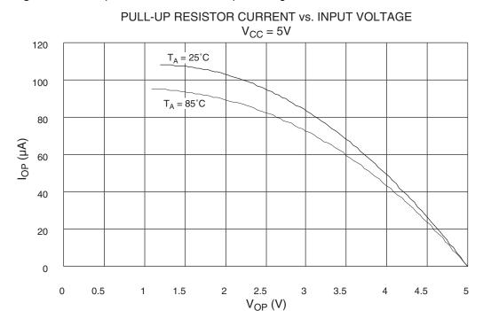
Figure 92. Pull-up Resistor Current vs. Input Voltage
