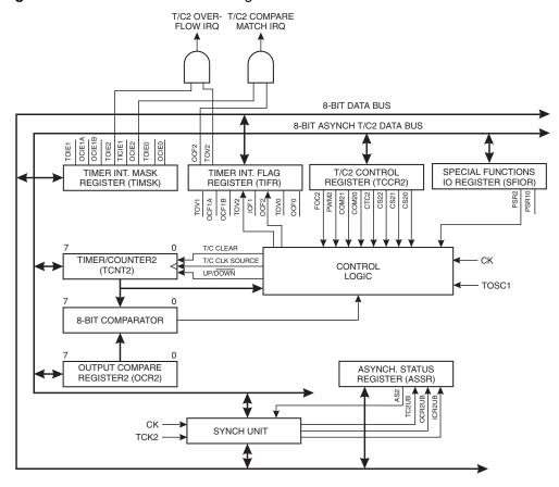
Figure 32. Timer/Counter2 Block Diagram
