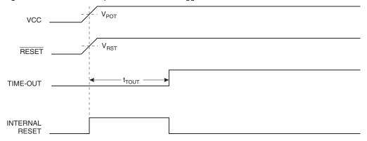
Figure 26. MCU Start-up, RESET Controlled Externally
