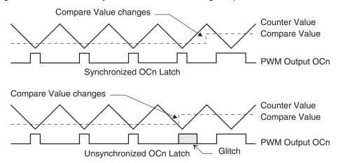
Figure 34. Effects of Unsynchronized OCR Latching in Overflow Mode.
