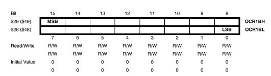
The Output Compare Registers are 16-bit read/write registers.
