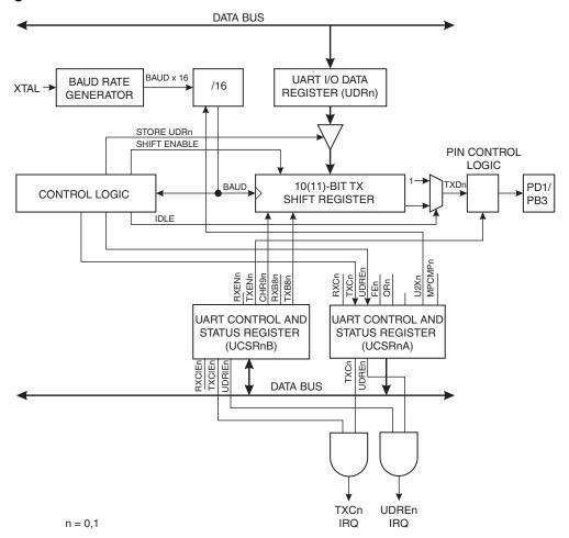
Data transmission is initiated by writing the data to be transmitted to the UART I/O Data Register, UDRn. Data is transferred from UDRn to the Transmit Shift Register when:
