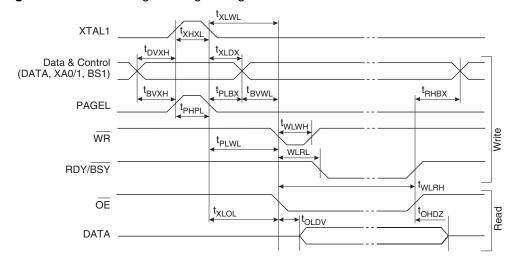
**Table 45.** Parallel Programming Characteristics,  $T_A = 25^{\circ}C \pm 10^{\circ}$ ,  $V_{CC} = 5V \pm 10^{\circ}(^{(1)(2)(3)})$
