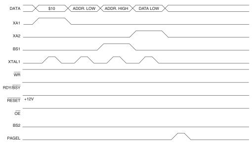
Figure 77. Programming the Flash Waveforms (Continued)
