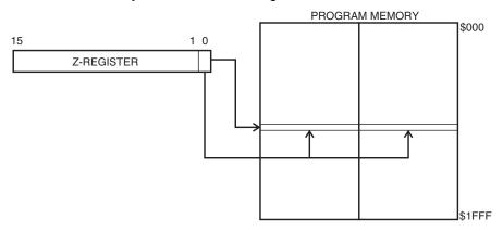
Constant byte address is specified by the Z-register contents. The 15 MSBs select word address (0 - 8K), the LSB selects Low byte if cleared (LSB = 0) or High byte if set (LSB = 1).
