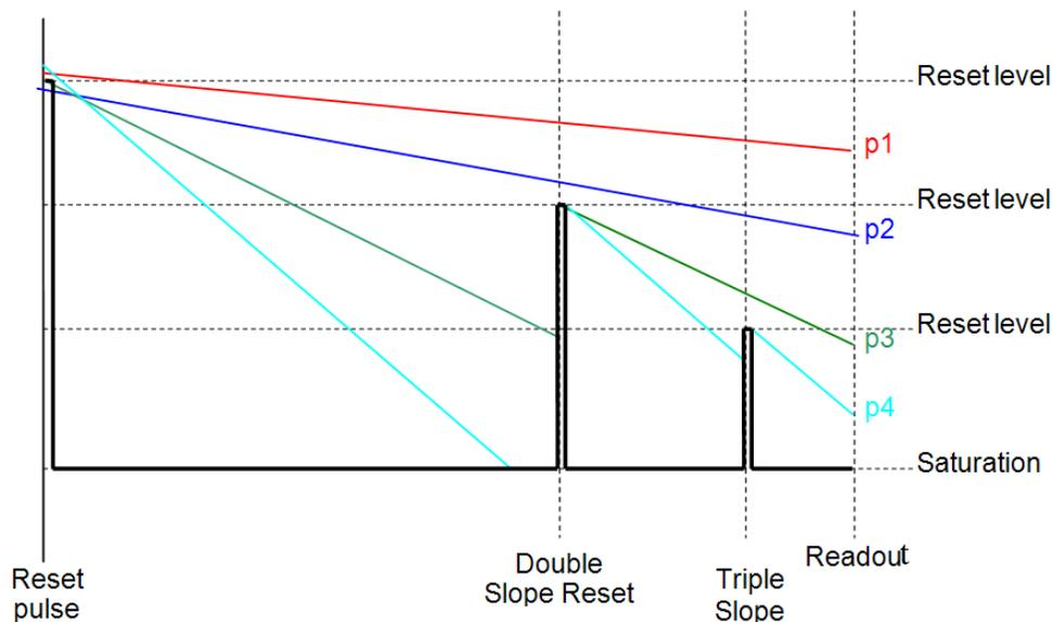
The reset levels are configured through external (power) pins. In master mode, the time stamps of the double and triple slope resets are configured in a method similar to configuring the exposure time. The time stamps are enabled through the registers seqmode1[5] and seqmode1[6], and their values are expressed in line or clock cycles in the registers reg\_tint\_ds\_timer and reg\_tint\_ts\_timer.
