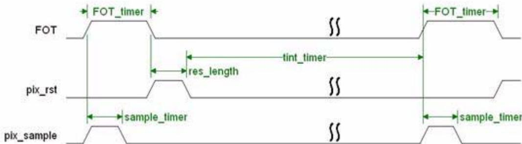
Ensure that the added value of the registers res\_length and tint\_timer always exceeds the number of lines that are read out. This is because the sequencer samples a new image after integration is complete, without checking if image readout is finished. Enlarging res\_length to accommodate for this has no impact on image capture.
