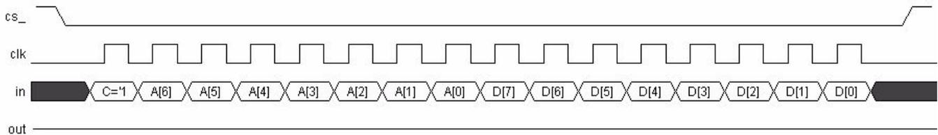
The 'out' line is held to High Z. The data for the address A is transferred from the shift register to the active register bank (that is, sampled) on a rising edge of cs\_n. Only the register block with address A can write its data on the 'out' bus. The data on 'in' is ignored.
