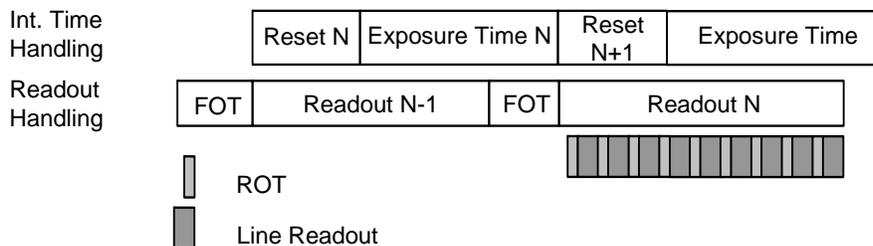
You have two options in the pipelined shutter mode. The first option is to program the reset and integration through the configuration interface and let the sequencer handle integration time automatically. This mode is called master mode. The second option is to drive the integration time through an external pin. This mode is called slave mode.
