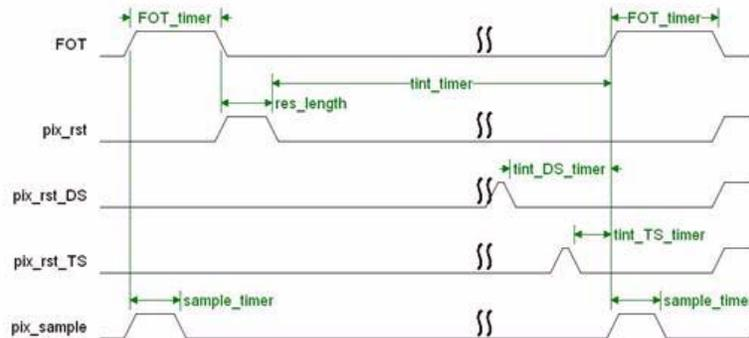
In slave mode, the values of res\_length, tint\_timer, tint\_DS\_timer, and tint\_TS\_timer in the configuration registers are ignored. You have full control through the pins int\_time, int\_time\_ds, and int\_time\_ts. You must configure the multiple slope parameters for the application and interpret the pixel data accordingly.
