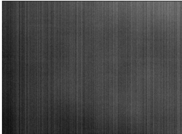
**Figure 24. Dark Image With FPN Correction Enabled (5x Amplified)**
