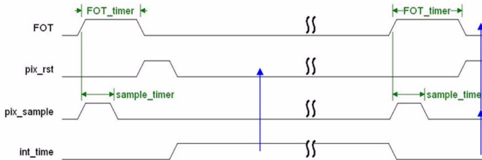
Changing a pixel's reset level during line readout might result in image artefacts during a small transient period. As a result, it is advised to only change the value of `int_time` during ROT.
