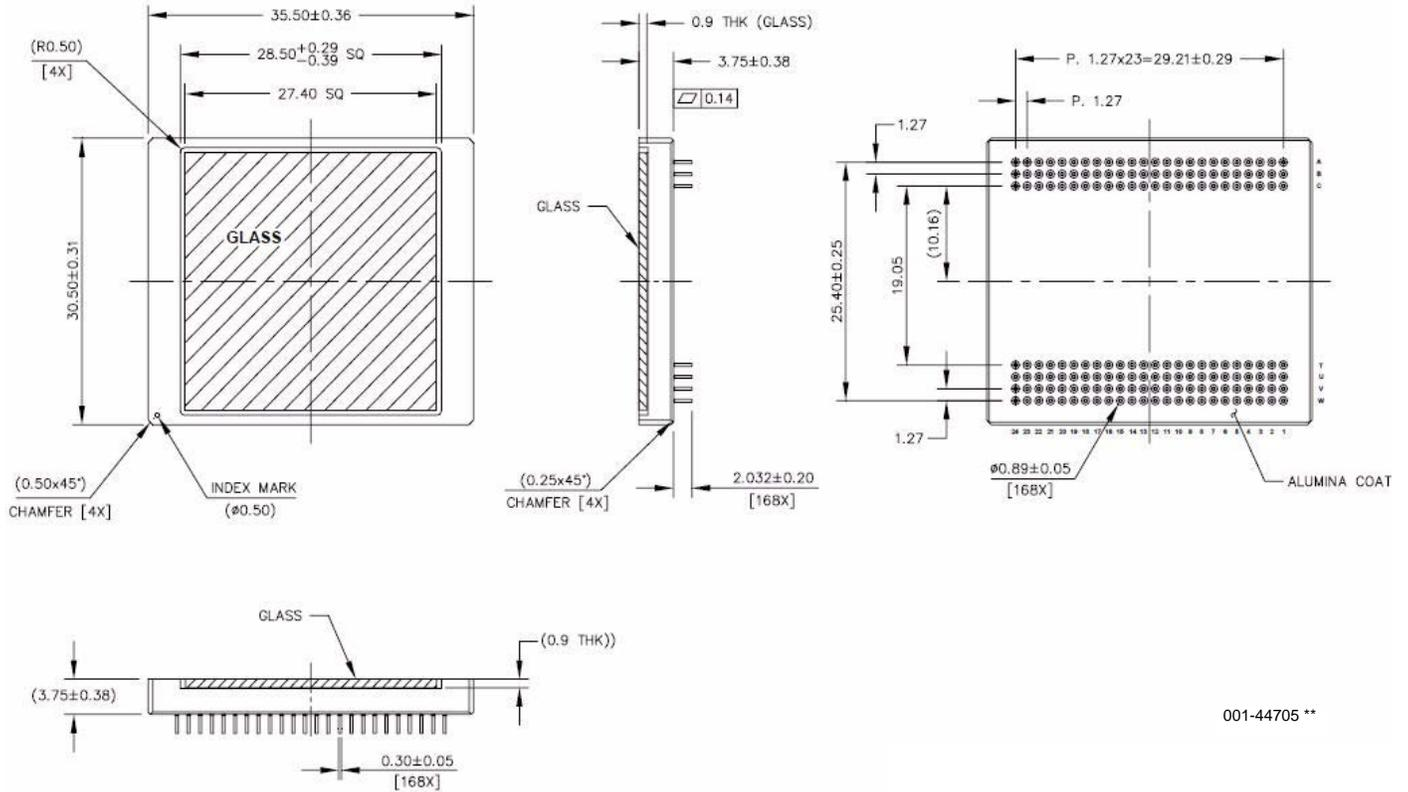
The total distance from the bottom of the  $\mu$ PGA package (same as the PCB plane) to the top of the die surface is 19.016 mm.
