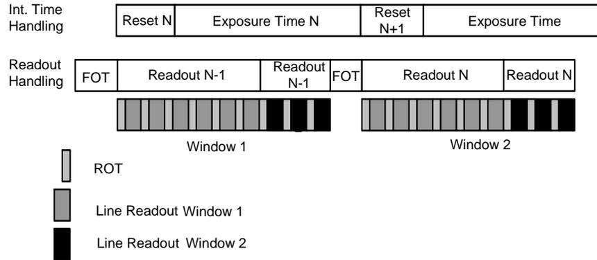
If the X size of the windows are not identical, the integration time in function of the number of lines read presents multiple slopes (proportional to the X size of these windows). Because this can cause confusion when programming the integration time, it is easier to configure all timer registers using the clock cycle configuration instead of the 'line' configuration.
