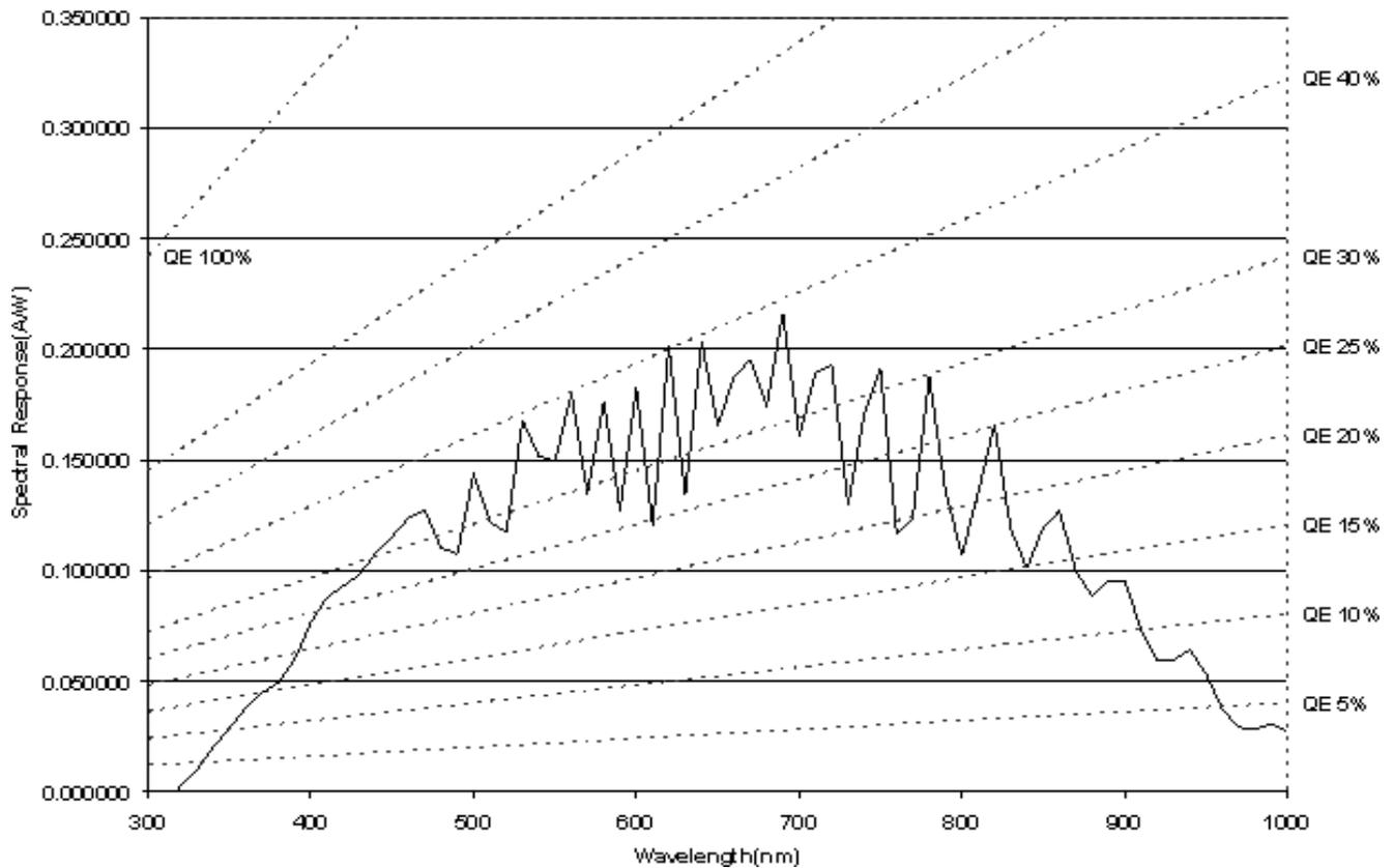
Figure 4. Spectral Response of LUPA 1300-2 Color Sensor
