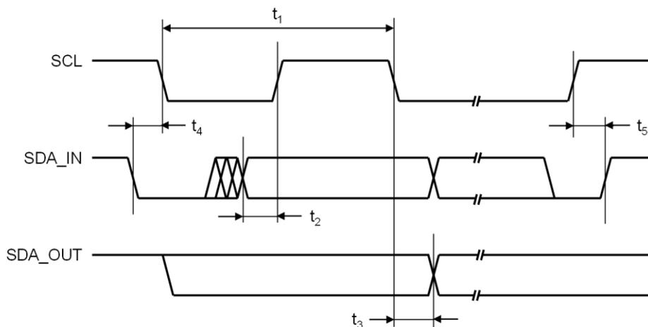
Figure 1. I<sup>2</sup>C Compatible Interface Timing
