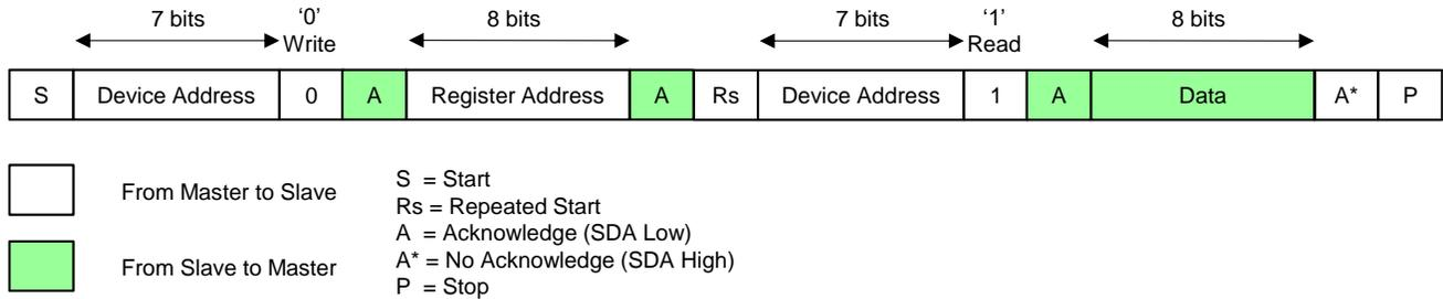
**Figure 6. I<sup>2</sup>C Read Cycle**
