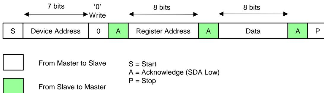
**Figure 5. I<sup>2</sup>C Write Cycle**
