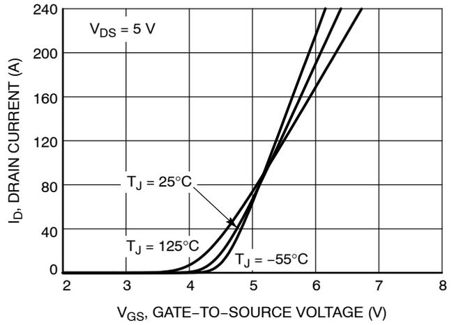
Figure 2. Transfer Characteristics
