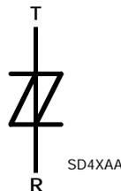
Terminals T and R correspond to the alternative line designators of A and B
