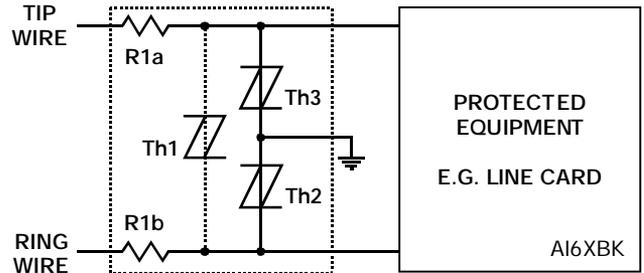
Figure 16. PROTECTION MODULE
