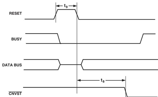
Figure 12. RESET Timing
