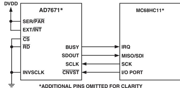
Figure 22. Interfacing the AD7671 to SPI Interface
