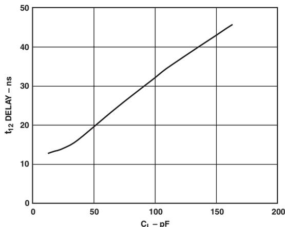
TPC 13. Typical Delay vs. Load Capacitance  $C_L$
