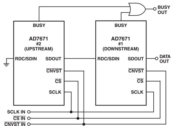
Figure 20. Two AD7671s in a Daisy-Chain Configuration
