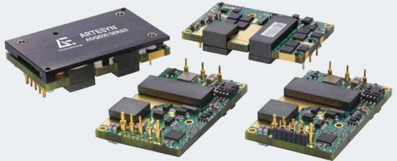
ADQ500 series quarter-brick isolated DC-DC converters produce a single fully regulated 12 V output. Rated at 500 watts, these converters can deliver up to 42 amps output current and have no minimum load requirement. They have an input voltage range of 36 to 75 V and are primarily designed for use with standard 48 V supplies in computing and server applications, as well as regulated 48V supplies in communications equipment.
