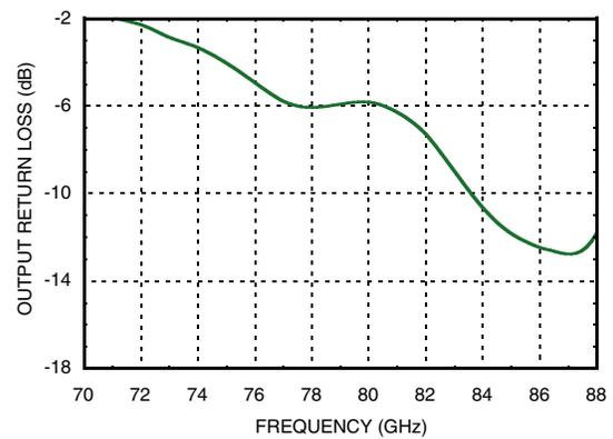
Note: Measured Performance Characteristics (Typical Performance at 25°C) Vdd1 = Vdd2 = 4V and Idd1 = 40mA, Idd2 = 90mA
