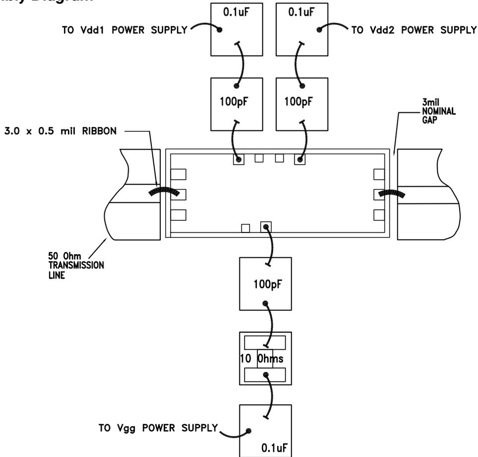
Note 1: Bypass caps should be 100 pF (approximately) ceramic (single-layer) placed no farther than 30 mils from the amplifier
