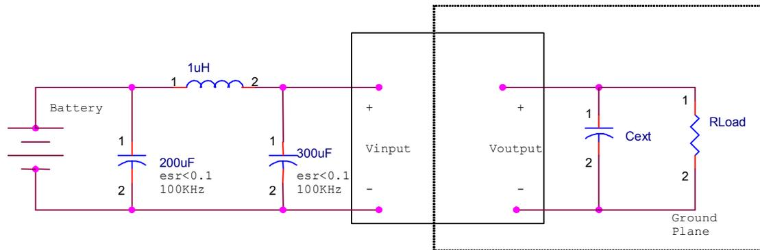
The input reflected ripple is measured with a current probe and oscilloscope. The ripple current is the current through the 1uH inductor.
