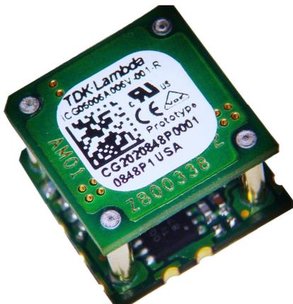
iCG power modules perform local voltage conversion from either a 5V or 12V bus. The iCG12006A007V utilizes a low component count that results in both a low cost structure and a high level of performance. The open-frame, compact, surface mountable design features a low profile and weight as well as additional edge plated pads that allow for extremely flexible and robust manufacturing processes.
