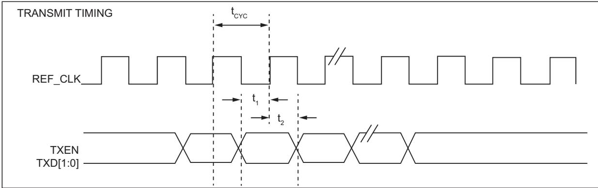
**FIGURE 7-2: RMII TIMING - DATA INPUT TO RMII**
