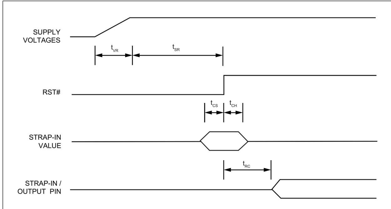
**TABLE 7-5: POWER-UP/RESET TIMING PARAMETERS**
