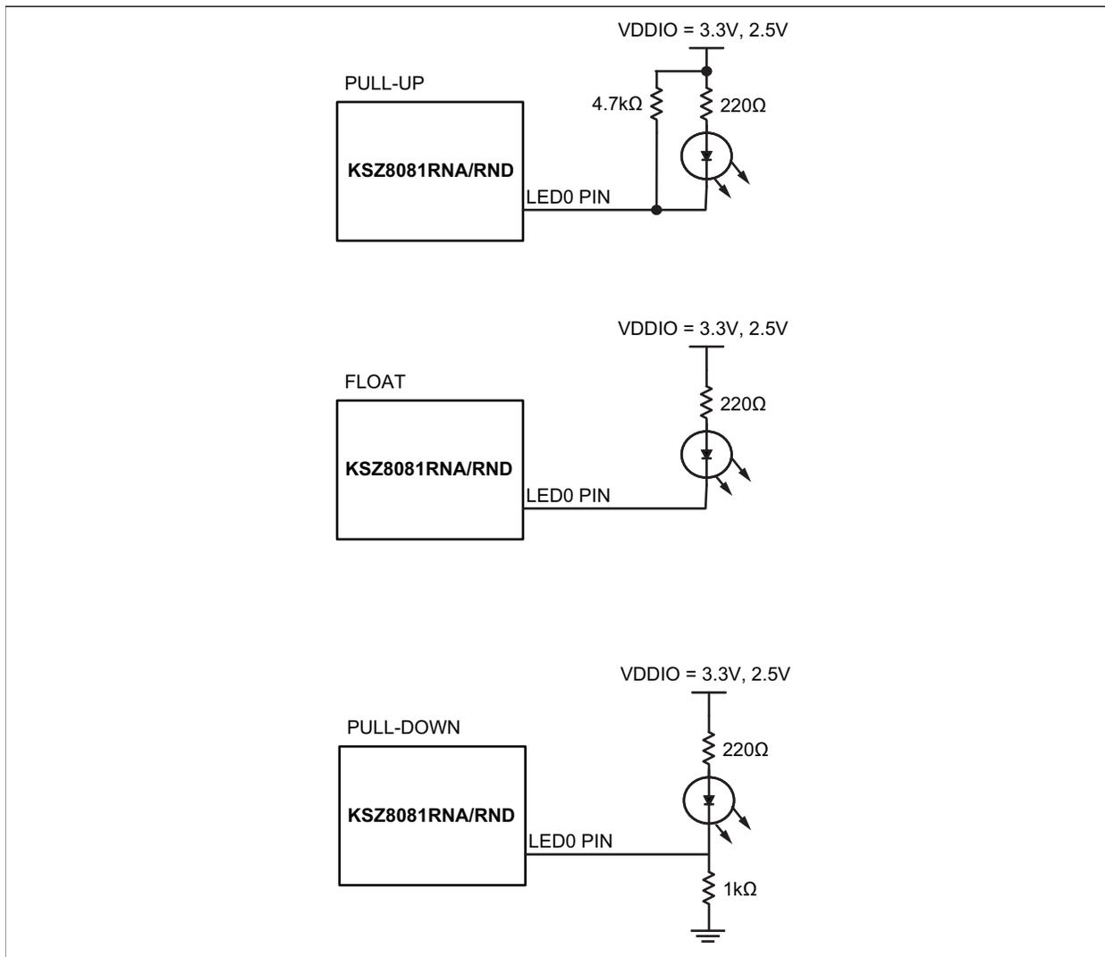
For 1.8V  $V_{DDIO}$ , LED indication support is not recommended due to the low voltage. Without the LED indicator, the ANEN\_SPEED strapping pin is functional with a 4.7 k $\Omega$  pull-up to 1.8V  $V_{DDIO}$  or float for a value of '1', and with a 1.0 k $\Omega$  pull-down to ground for a value of '0'.
