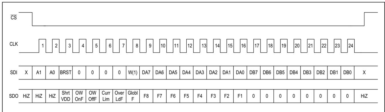
Figure 12. Addressed SPI Two Byte Write Command
