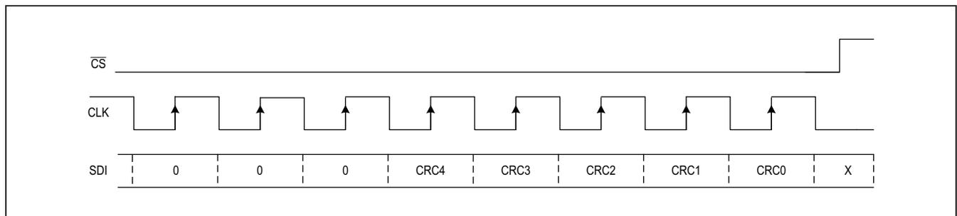
Figure 19. FCS Byte Expected from the SPI Master
