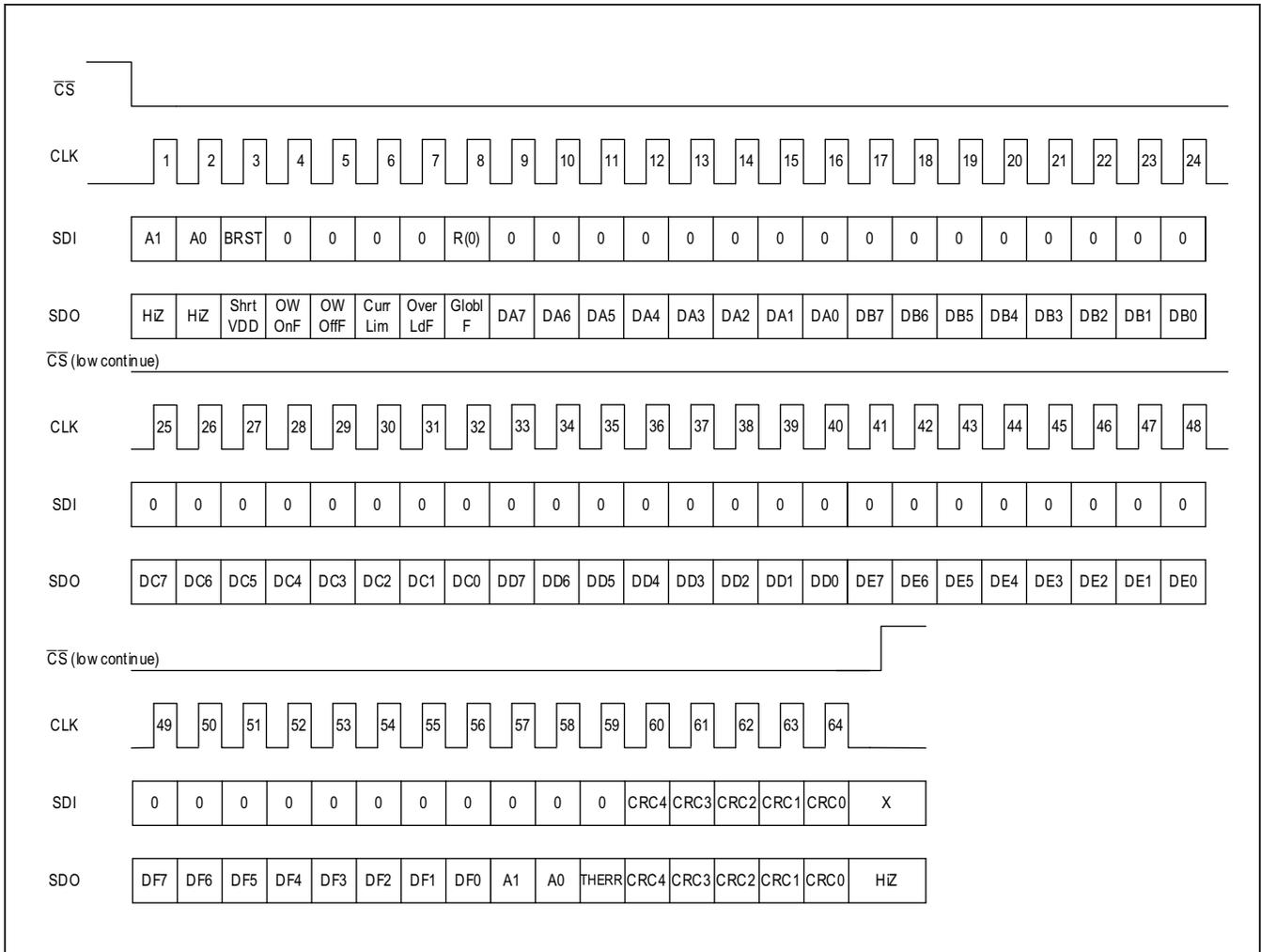
Figure 16. Addressed SPI Burst Read Command with CRC
