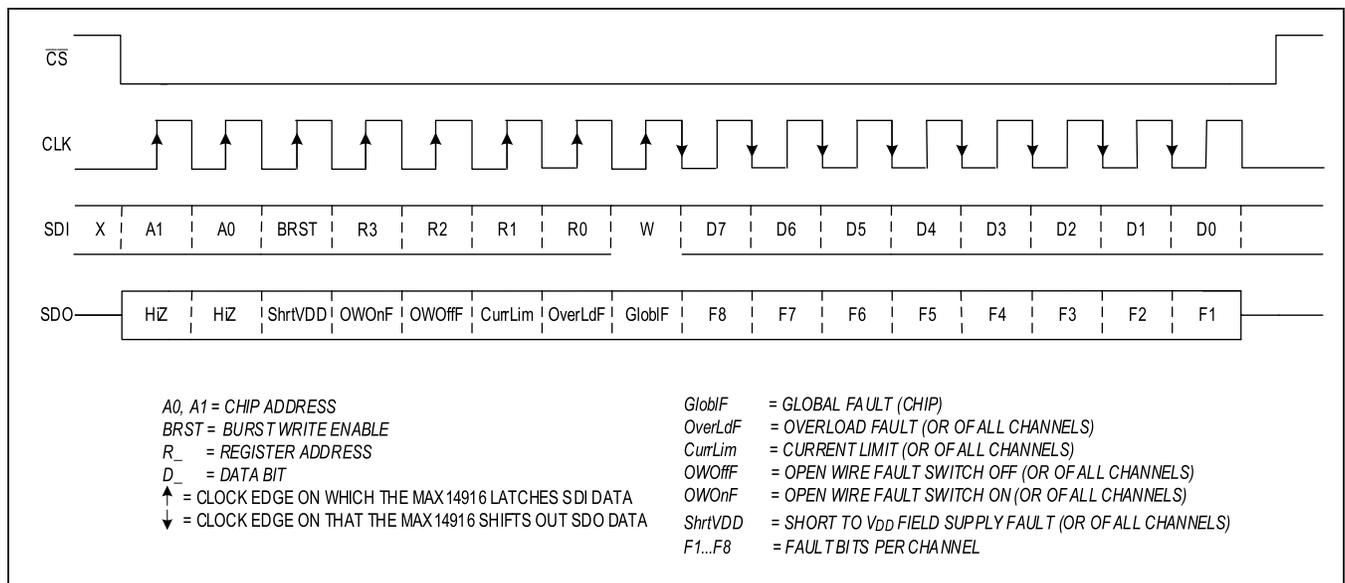
Figure 11. Addressed SPI Single Cycle Write Command
