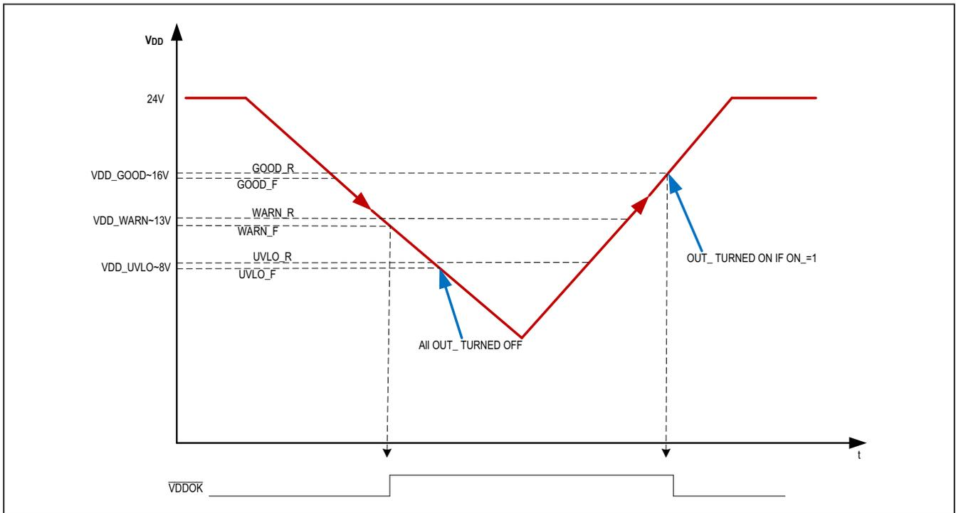
Figure 4. V<sub>DD</sub> Monitoring with VDDOnThr = 1
