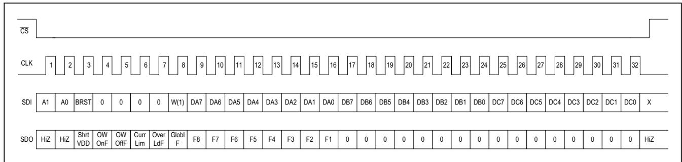
Figure 13. Addressed SPI Three Bytes Burst Write Command
