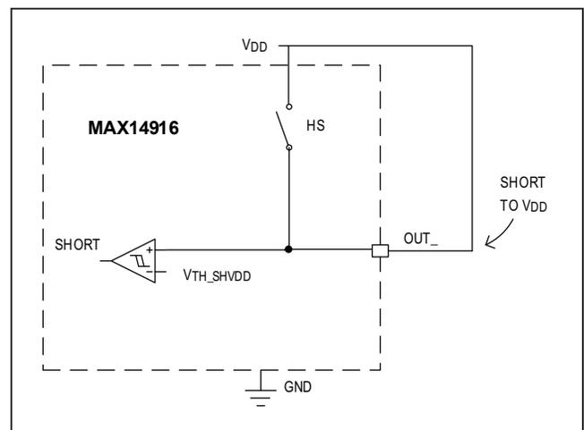
Figure 6. Short to V<sub>DD</sub> Detection Scheme
