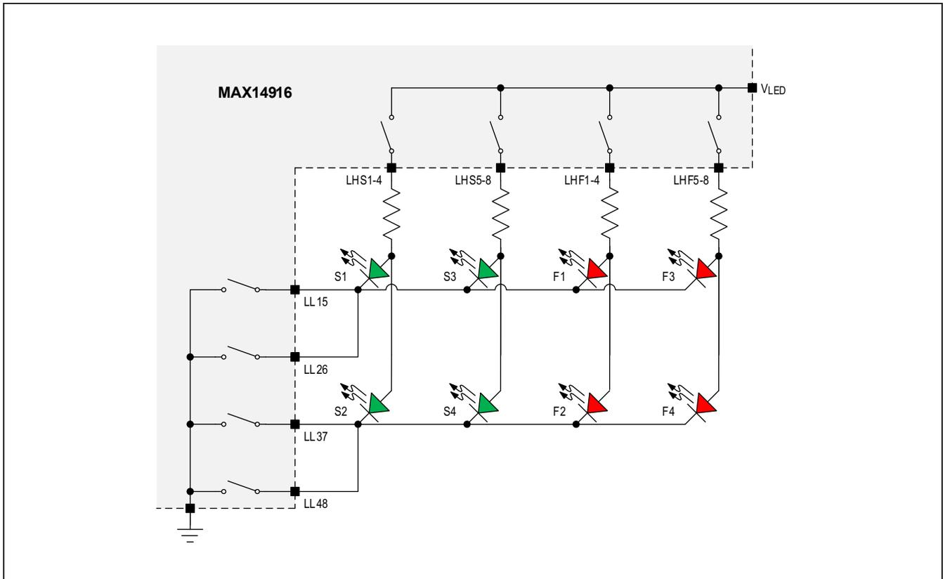
Figure 9a. LED Matrix Scheme for Quad Configuration
