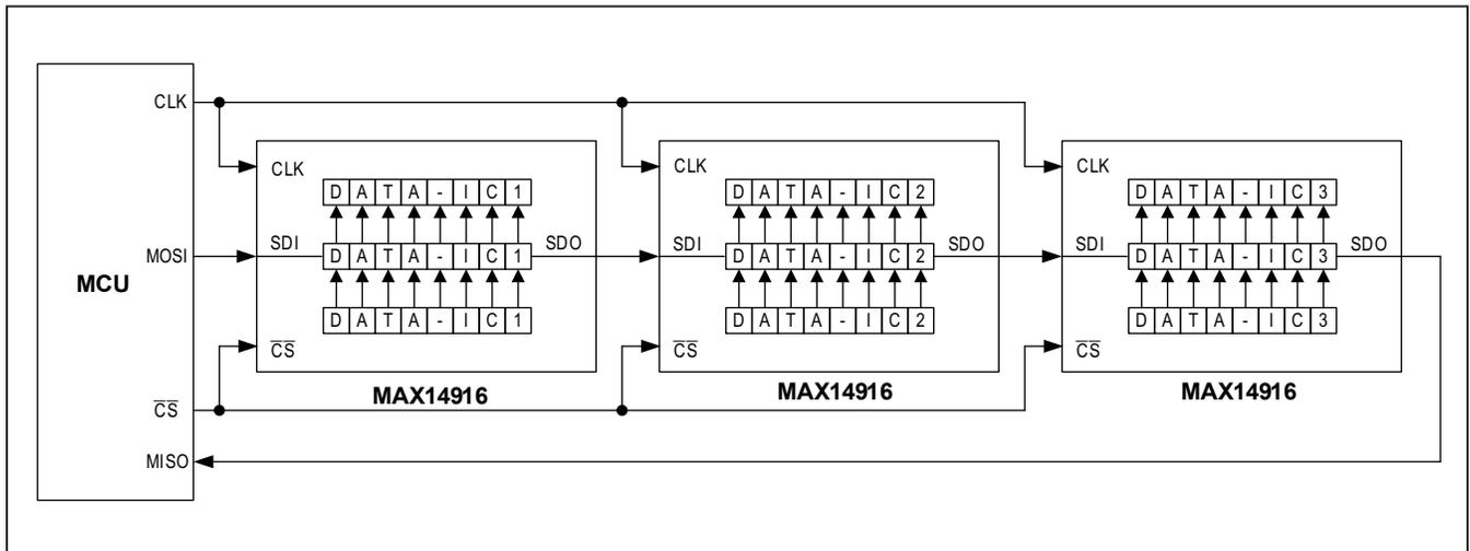
Figure 17. Daisy-Chaining Diagram of Three MAX14916
