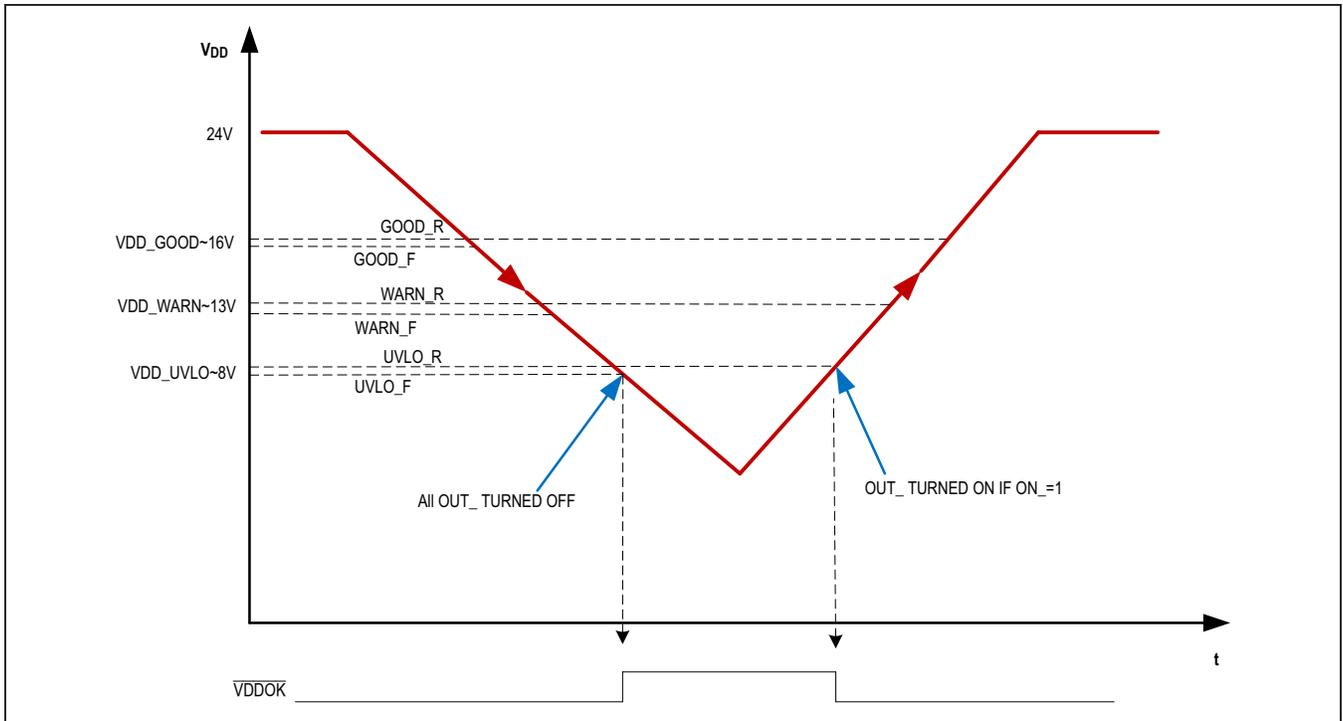
Figure 3. V<sub>DD</sub> Monitoring with VDDOnThr = 0
