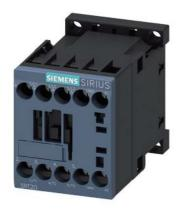
Contactor, 5 HP, 460 / 575 V, 1 NO, 208 V AC, 50 / 60 Hz, 3-pole, Size S00 screw terminal
