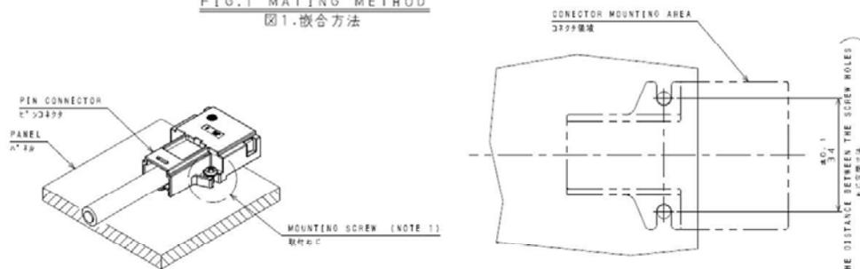
FIG. 2 PANEL MOUNTING METHOD
