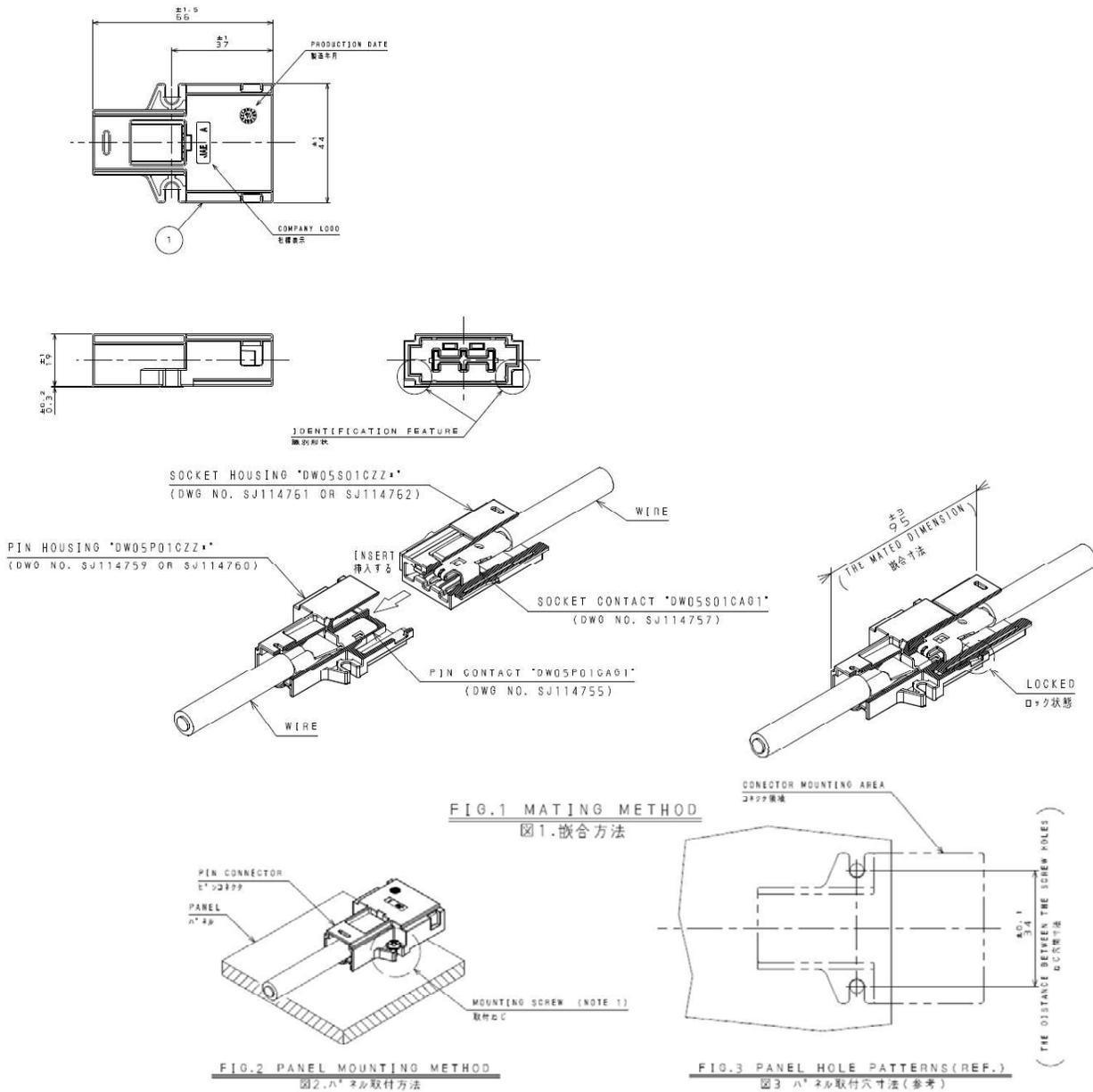
NOTE 1.RECOMMENDATION MOUNTING SCREW IS CROSS RECESSED HEAD SCREW.
