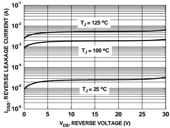
Figure 26. SyncFET<sup>™</sup> Body Diode Reverse Leakage vs. Drain-Source Voltage
