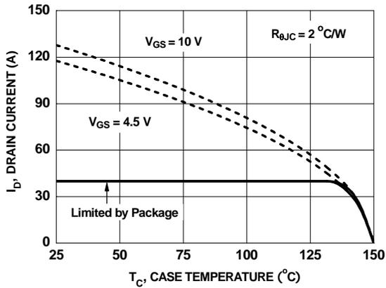
**Figure 21. Maximum Continuous Drain Current vs Case Temperature**
