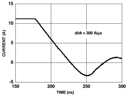
Figure 25. FDMS7600AS SyncFET<sup>™</sup> Body Diode Reverse Recovery Characteristic
