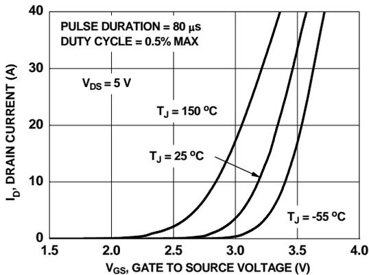
Figure 5. Transfer Characteristics
