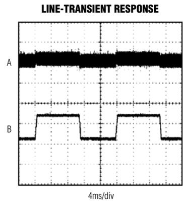
$V_{OUT} = 5\text{V}$ , LOAD CURRENT = 1A
