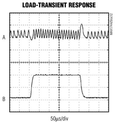
$V_{IN} = 7.2\text{V}$ ,  $V_{OUT} = 3.3\text{V}$ , LOAD CURRENT = 0.1A TO 2A
