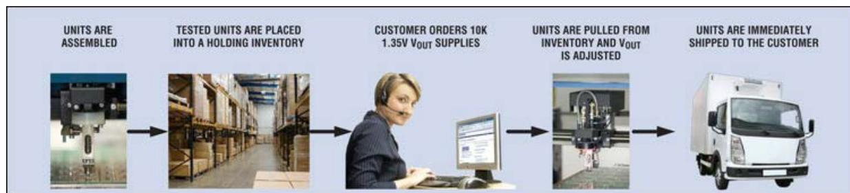
Figure 2. Illustrating the manufacturing benefits of using an E<sup>2</sup>CRef.
