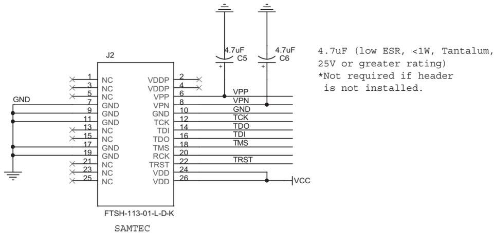
The programming header is optional. It provides a means for re-programming the chip on board if necessary.
