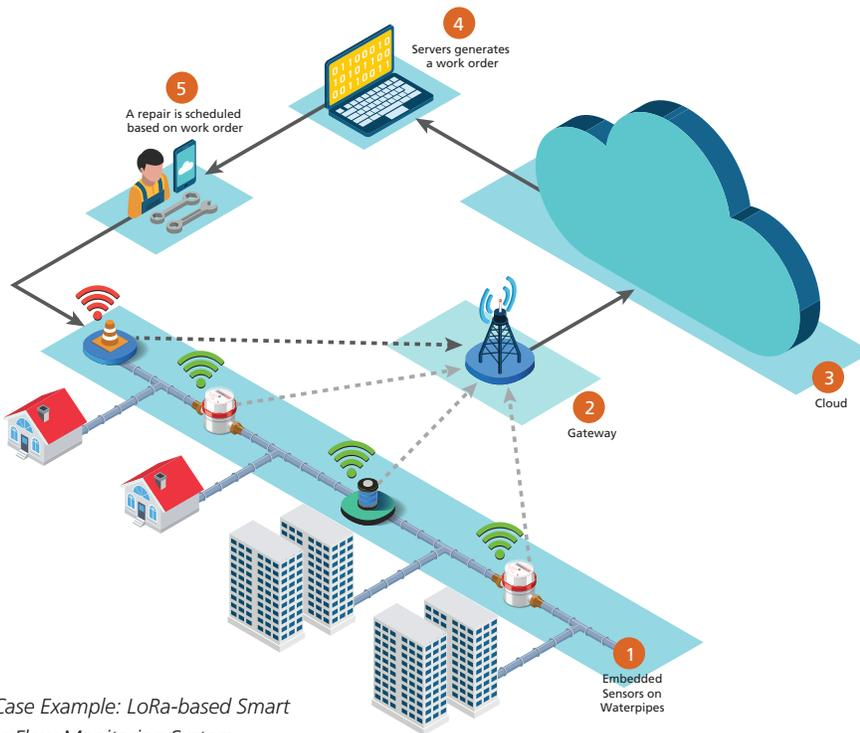
Use Case Example: LoRa-based Smart Water Flow Monitoring System
