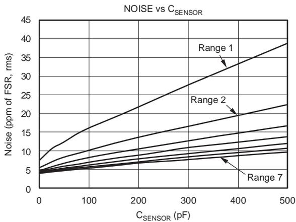
NOISE vs  $C_{\text{SENSOR}}$
