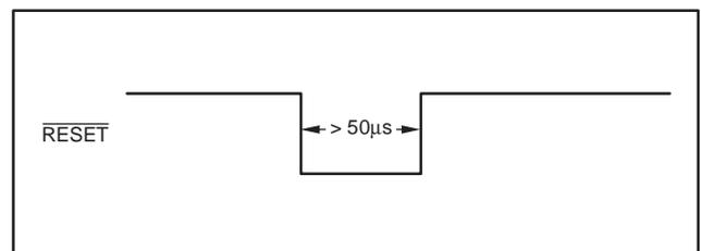
Figure 9. Reset Timing
