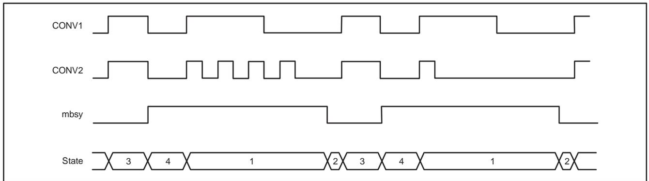
**Figure 16. Equivalent CONV Signals in Non-Continuous Mode**
