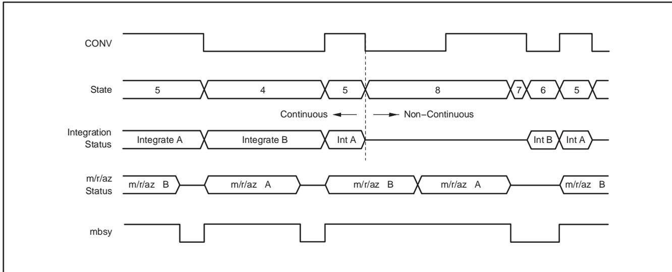
Figure 18. Changing from Continuous Mode to Non-Continuous Mode
