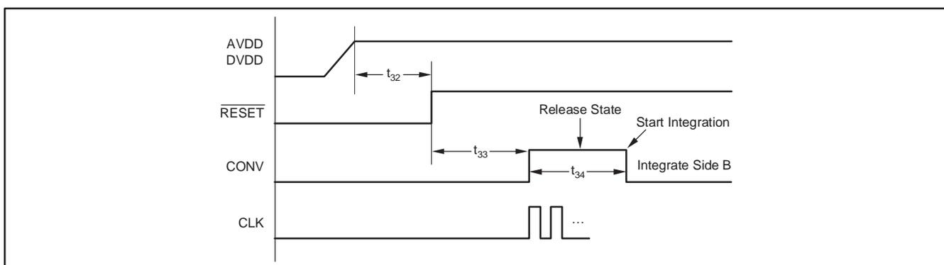
Figure 28. Timing Diagram at Power-Up of the DDC114
