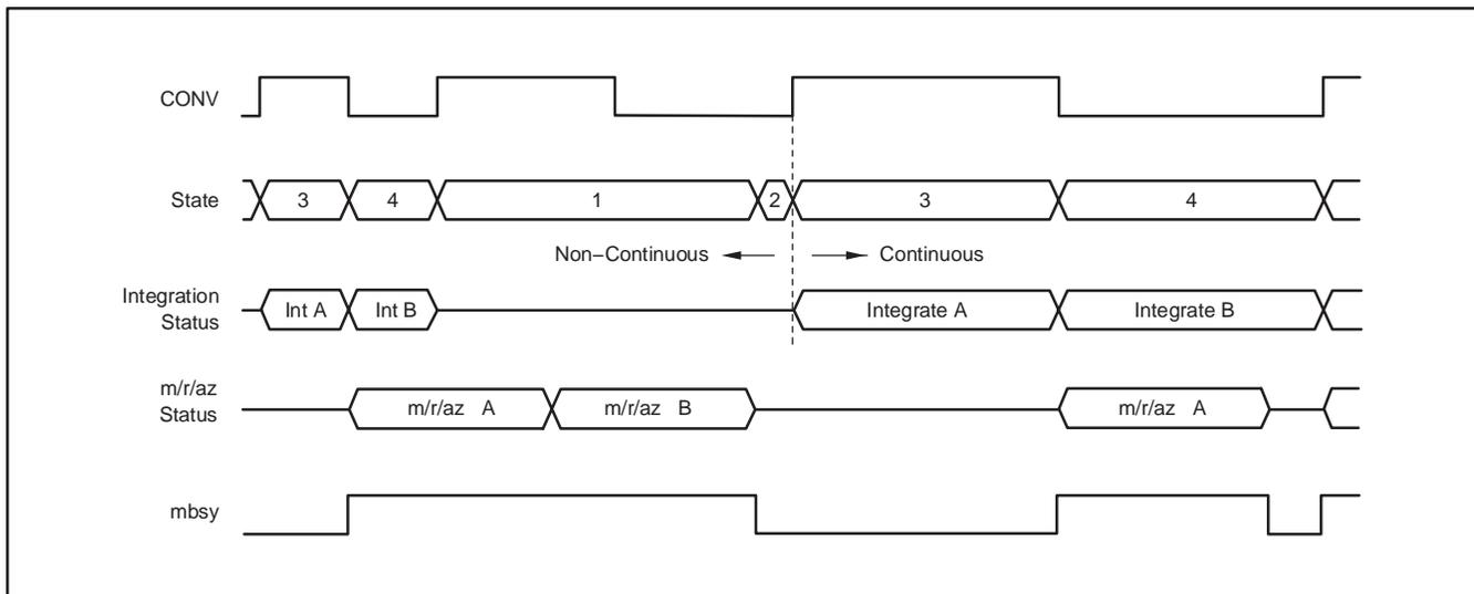
Figure 19. Changing from Non-Continuous Mode to Continuous Mode
