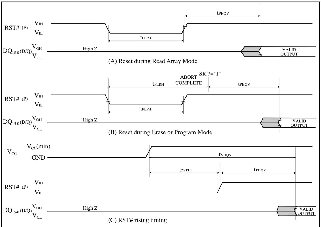
Figure 8. AC Waveform for Reset Operations
