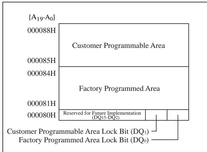
Figure 3. OTP Block Address Map for OTP Program
