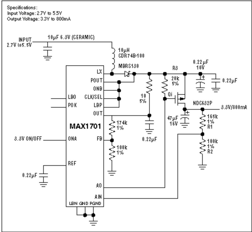
Figure 1. This buck/boost circuit assumes the buck (linear regulator) mode for inputs above 3.3V and the boost (switching regulator) mode for inputs below 3.3V.
