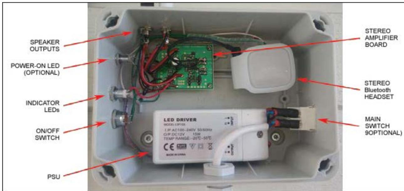
Figure 7. The system assembled in an enclosure.
