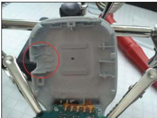
*Figure 2. Headset front cover, inside view.*
