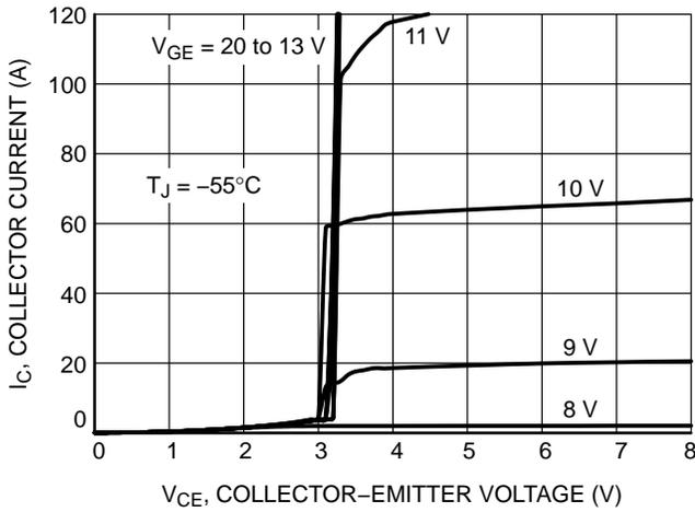
Figure 3. Output Characteristics
