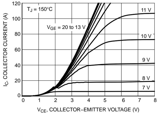
Figure 2. Output Characteristics
