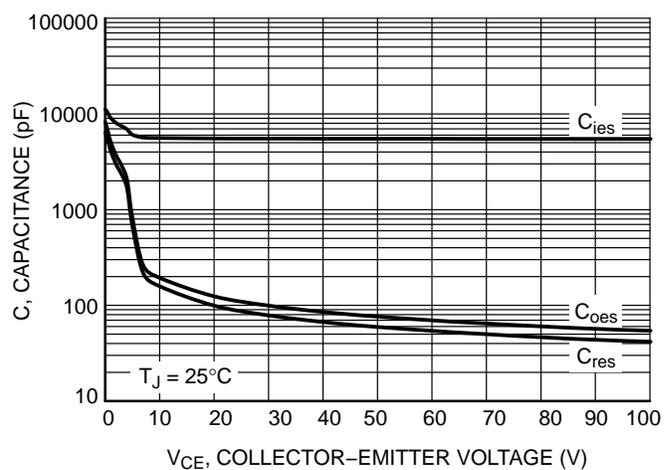
Figure 6. Typical Capacitance
