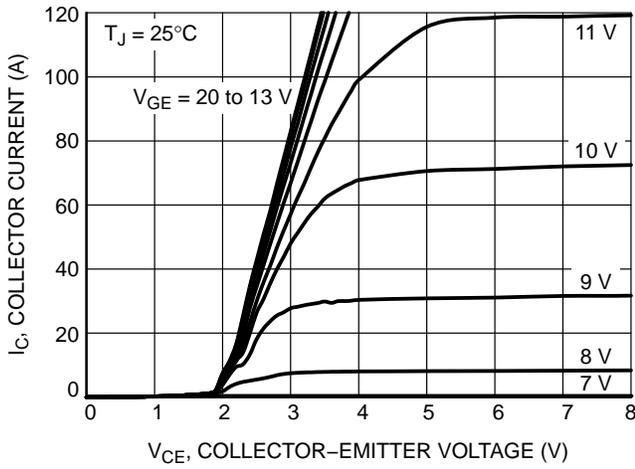
Figure 1. Output Characteristics
