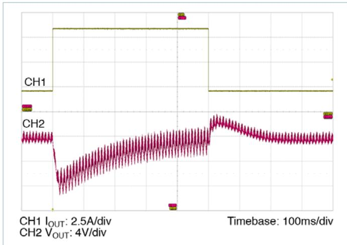
**Figure 7** — Typical output voltage transient response,  $T_{CASE} = 30^{\circ}C$ ,  $V_{IN} = 230V$ ,  $I_{OUT} = 8.3A$ ,  $2.1A$
