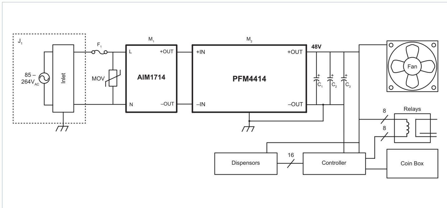
The PFM in a VIA package is available in chassis-mount option, saving the cost of a PCB and allowing access to both sides of the power supply for cooling. The parts list below minimizes the number of interconnects required between necessary components, and selects components with terminals traditionally used for point-to-point chassis wiring.
