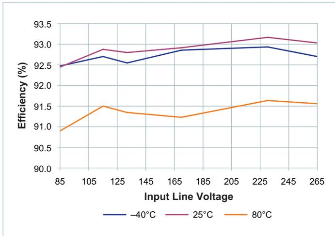
Figure 1 — Full load efficiency vs. line voltage
