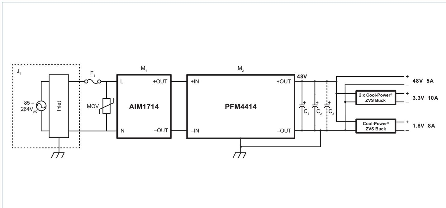
The PCB terminal option allows mounting on an industry standard printed circuit board, with two different pin lengths. Vicor offers a variety of downstream DC-DC converters driven by the 48V output of the PFM in a VIA package. The 48V output is usable directly by loads that are tolerant of the PFC line ripple, such as fans, motors, relays, and some types of lighting. Use downstream DC-DC point-of-load converters where more precise regulation is required.
