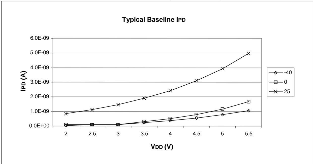
**FIGURE 14-2: TYPICAL IPD vs.  $V_{DD}$  OVER TEMP (+85°C)**
