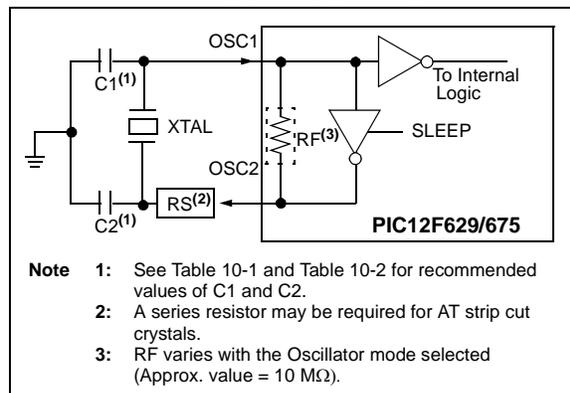
**FIGURE 10-2: EXTERNAL CLOCK INPUT OPERATION (HS, XT, EC, OR LP OSC CONFIGURATION)**
