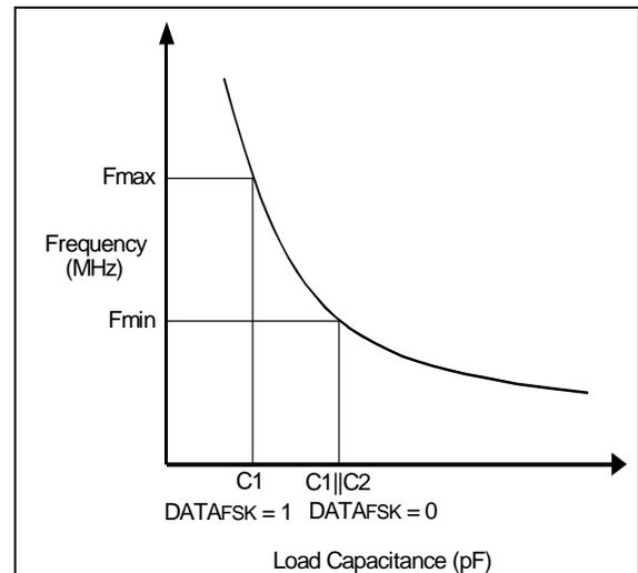
**TABLE 9-3: TYPICAL TRANSMIT CENTER FREQUENCY AND DEVIATION (FSK MODE) <sup>(1)</sup>**
