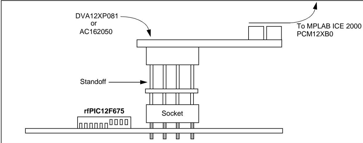
**FIGURE 10-17: IN-CIRCUIT PROGRAMMING USING THE PARALLEL DIP SOCKET**
