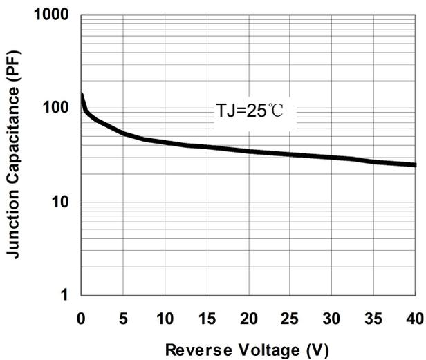
Fig.1-Typical Junction Capacitance
