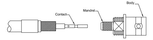
3) Insert the contact into the body and ensure that the contact captivates. Make sure the braid is on the outside of the mandrel. Slide the ferrule over the braid until the ferrule butts up against the body. Crimp the ferrule using the correct tool the the connector.
