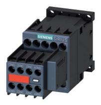
Power contactor, AC-3 9 A, 4 kW / 400 V 2 NO + 2 NC, 110 V AC, 50 Hz 120 V, 60 Hz, with plugged on varistor, 3-pole, Size S00 Screw terminal Captive auxiliary switch
