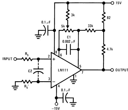
Pin connections shown are for LM111H in the LMC0008C package
