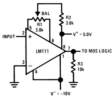
Figure 33. Zero Crossing Detector Driving MOS Logic
