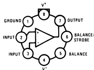
Note: Pin 4 connected to case
