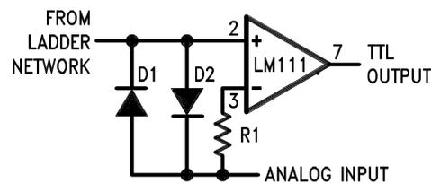
Figure 38. Using Clamp Diodes to Improve Response
