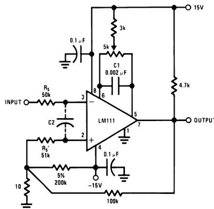
**Figure 24. Positive Feedback with High Source Resistance**
