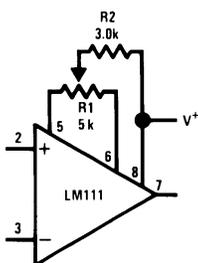
Figure 25. Offset Balancing
