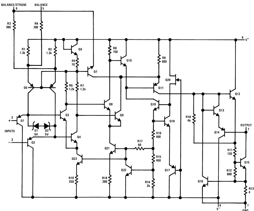
Pin connections shown on schematic diagram are for LMC0008C package.
