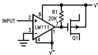
**Figure 34. Zero Crossing Detector Driving MOS Switch**
