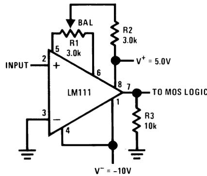
Figure 45. Zero Crossing Detector Driving MOS Logic
